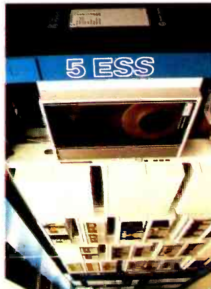
AT&T'S 5ESS SYSTEM, USING THE MOST advanced local digital switch, meets today's needs, and can expand to meet tomorrow's demands—including ISDN's three operating modes. The system's 5ESS switching module is shown above, including a test circuit that monitors communication with other modules over light-wave links.
