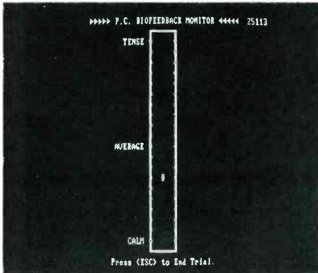
FIG. 6—THE CALMER YOU GET the lower the indicator's position, and the lower the tone heard from the speaker.
