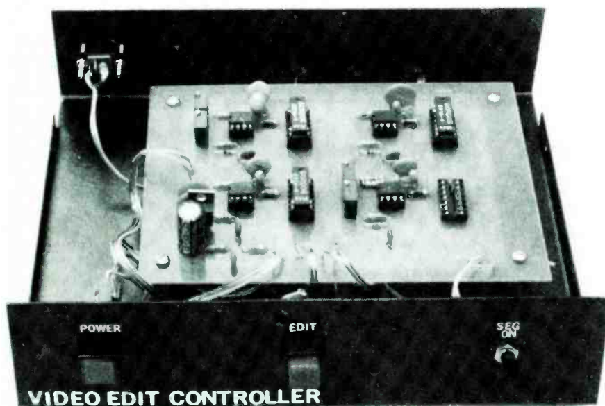
FIG. 3—THE PRINTED-CIRCUIT BOARD is mounted in the cabinet using spacers at each mounting screw. Make certain that there is some kind of wire between the PC board's ground trace and the metal cabinet.
