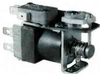
FIG. 8—THIS LATCHING RELAY, the 589R from Potter and Brumfield, flips a mechanical toggle from side to side like a mechanical flip-flop, changing state when the coil is activated by a pulse.
