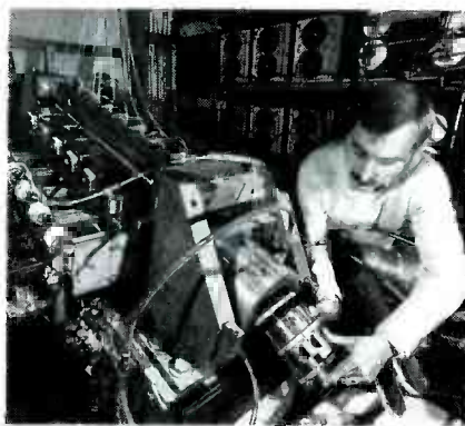
SANDIA EXPERIMENTER Ronald Kaye inserts a projectile into the breech of a six-stage electromagnetic launcher, which is being developed as a possible alternative to rockets for frequent launches of small payloads.
