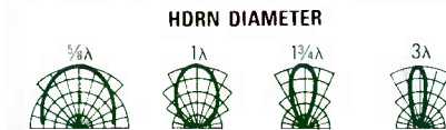
FIG. 7—AS HORN MOUTH SIZE increases relative to wavelength, directivity increases, since audio wavelength is comparable to mouth size. Shown are directional patterns of decreasing beamwidth, for four horn diameters relative to \lambda .
