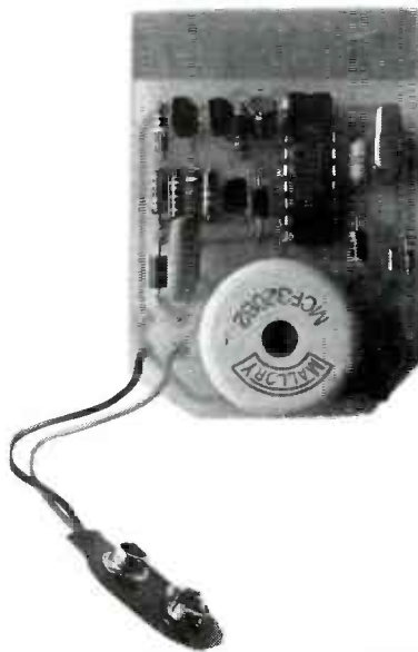
FIG. 7—A FINISHED ALERT MODULE. It can plug into any ordinary phone jack; use a T-connector if you must connect both a phone and an alert module to the same jack.
