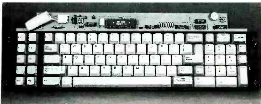
FIG. 1—A PC KEYBOARD is a small computer in itself. This keyboard's circuitry is based on an 8048 microcontroller that's specifically designed to handle and control I/O.
