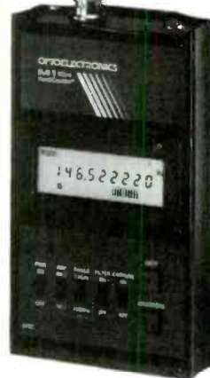
Shown with optional TA100S antenna—Actual frequency measurement shown (not simulated).
