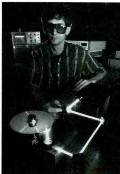
IBM SCIENTIST Dr. William J. Kozlovsky demonstrates a blue-laser that writes and reads data on a removable magneto-optical disk at a world-record density of 2.5 gigabits per square inch.
