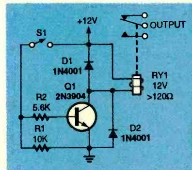
FIG. 12—TRANSISTOR-DRIVEN RELAY with a coil damper.
