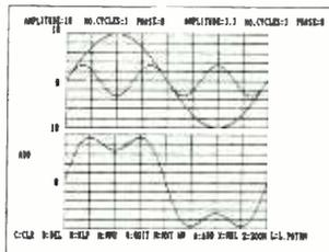
Figure 1. Addition of Sine Waves
