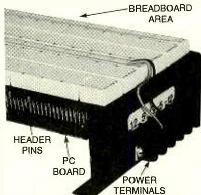
FIG. 6—CLOSE-UP VIEW OF J2, the circuit board, chassis, and breadboard strips.
