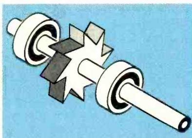
**FIG. 1—THE \$14 ORALSAFE DENTAL handpiece can be cut down to provide an air turbine the size and mass of a plotter pen. Air blown tangentially across the nylon pawl rotates the hollow shaft at extremely high speeds.**
