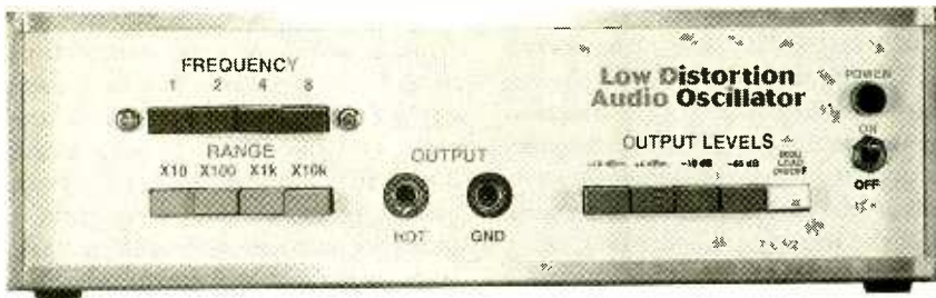
FIG. 2—HERE'S THE FRONT-PANEL layout for the instrument. The frequency and range selector switches discussed are on the left-hand side.
