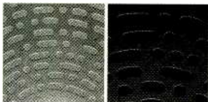
Fig. 1 One way that DVDs squeeze more data on a disk is to space the lands and pits that contain the data much tighter. The spacing for a DVD disk is shown on the left; that for a standard CD on the right.
