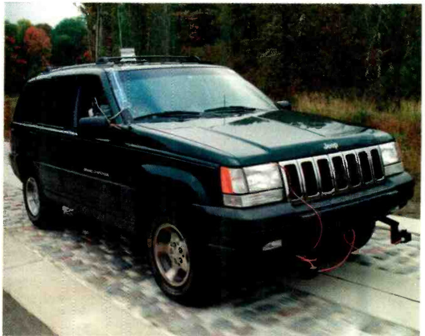
THE CHRYSLER AUTOMATED DURABILITY ROAD has a guidance wire embedded in the road. Twin inductive coil sensors temporarily mounted on the front of the vehicle measure pick up frequencies from the wire (Chrysler Corporation).
