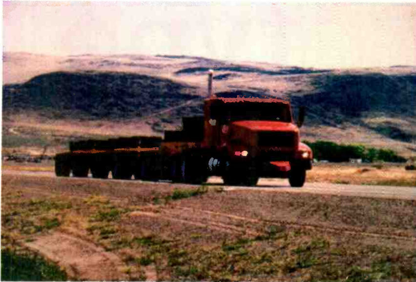
ONE OF THE DRIVERLESS TRUCKS circling the WesTrack for pavement testing (Nevada Automotive Test Center).
