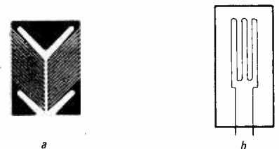
FIG. 5—STRAIN GAGES can be made from foil (as in a) or from wire (as in b)
