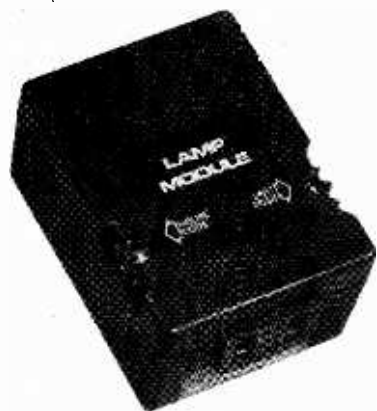
FIG. 9—THE BSR LAMP-CONTROL MODULE. The house and unit codes are easily set using thumbwheel switches.
