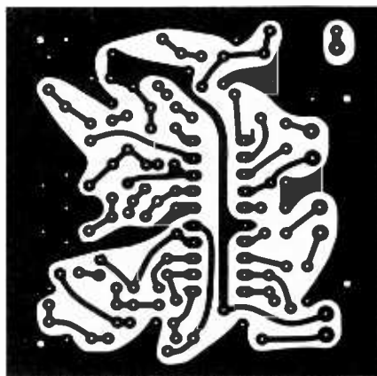
FIG. 5—HERE IS A FULL-SIZE foil diagram of the single-sided decoder board.
