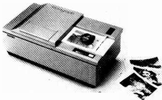
FIG. 4—THE MAVIGRAPH PRINTER can produce a color print from the Mavica or other still-video source in about five minutes.
