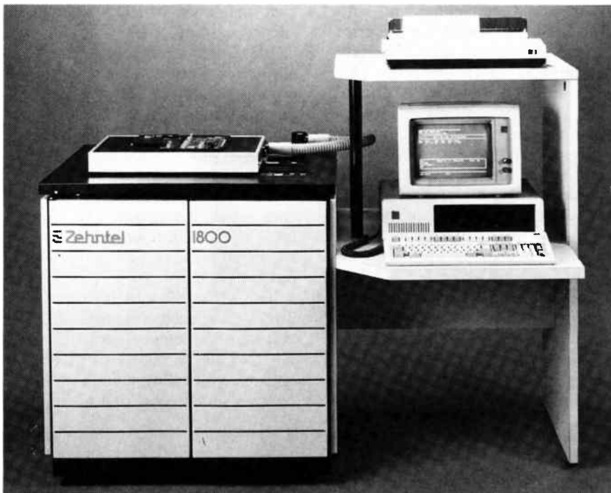
FIG. 4—ZEHNTTEL 1800 BOARD TESTER. A PC serves as controller, and the UUT fixture is on the console at left. Note the vacuum hose to the right. The 1800 is prewired for 640 analog/digital test points.
