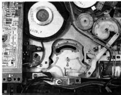
FIG. 6—A TYPICAL LOADING GEAR train is usually covered by a protective plastic guard that must be removed for servicing. This gear train is on the bottom of the chassis.
