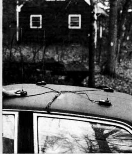
FIG. 6—DIRECTION FINDING using Doppler System's four matched quarter-wave whips, shown in (a), are supported on magnetically mounted bases for mobile operation. In (b), four collapsible antennas are mounted on a sturdy platform, on top of the author's roof.
