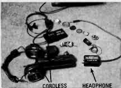
FIG. 4—USE THE AUTHOR'S home-built adaptor box with either a pair of stereo headphones, or a cordless infrared transmitter and receiver.
