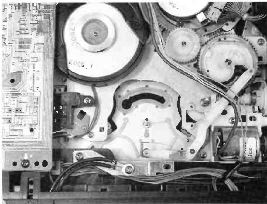
FIG. 4—A TYPICAL LOAD MOTOR is located on the bottom side of the VCR's chassis.
