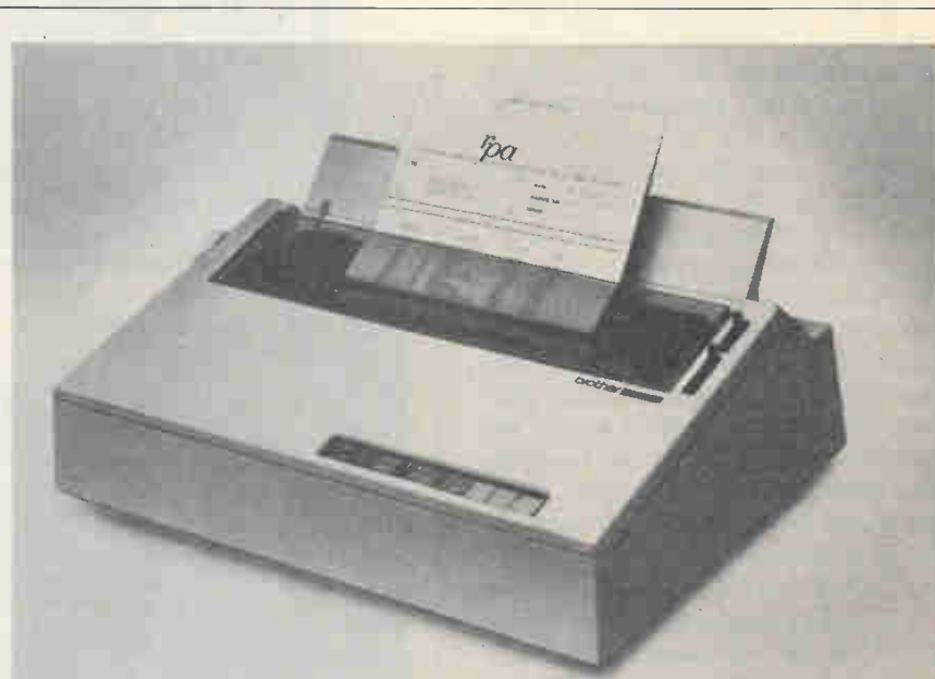
A compact, neat-package appearance is seen in the Brother HR-15 daisy-wheel printer. Latest versions can handle the underscore from word processors.
