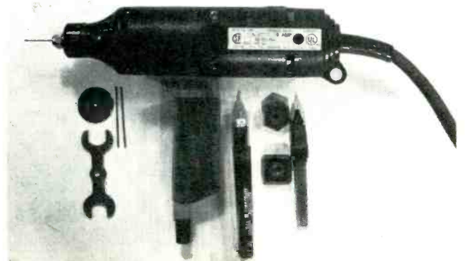
FIG. 1—TINTED SHELLAC, a FapiJog etch pen, a high-speed rotary drill, and drill bits are the only tools you need to make high-quality PC boards.
