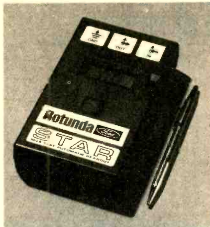
FIG. 3—SELF-TEST AUTOMATIC READOUT, or STAR, translates a diagnostic pulse string into an easily read fault code.
