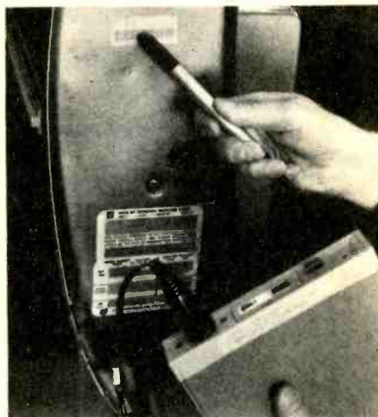
FIG. 4—THE VIN (Vehicle Identification Number) can be written as a bar code that may be read by a portable data terminal.
