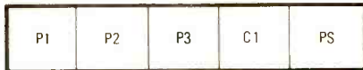
FIG. 12—FIVE-BYTE PREFIX carries information for multiplexing and error detection, and describes the data group that follows.
