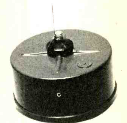
FIG. 7—A COMMON SEWING NEEDLE is used as the electron-emission source. The blunt end of the needle is soldered to the anode of the rectifier.
