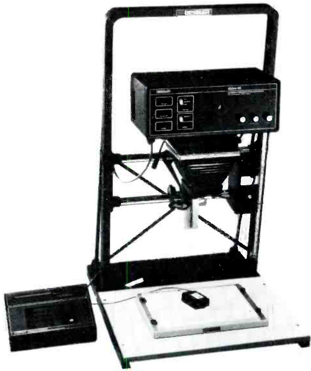
FIG. 5—BESELER's DICHO 45 enlarging system is programmable by means of plastic cards with magnetic stripes.
