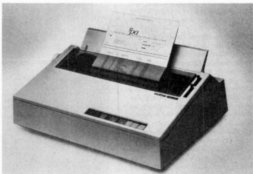
A compact, neat-package appearance is seen in the Brother HR-15 daisy-wheel printer. Latest versions can handle the underscore from word processors.
