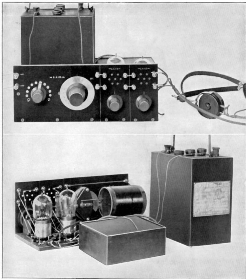
Fig. 3. Front and rear views of a complete receiving outfit employing the universal tuner
