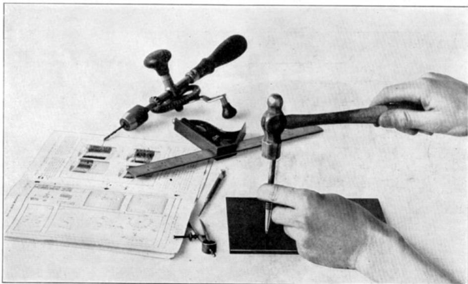
Fig. 3. Punch mark makes accurate drilling easier
