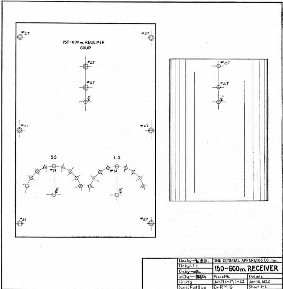
Fig. 4. Scale drawing of panel and tube, reduced to one half size
