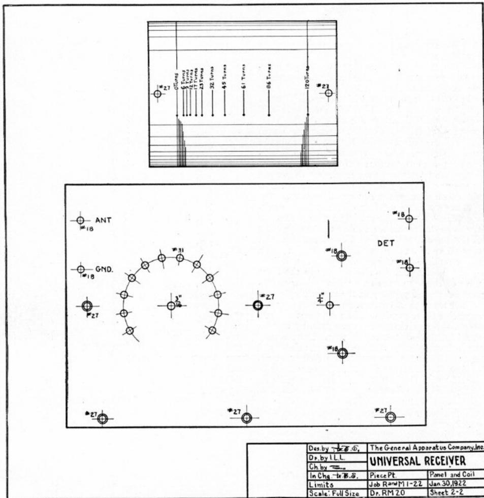
Fig. 5. Scale drawing of coil details and panel lay-out, reduced to one half size
