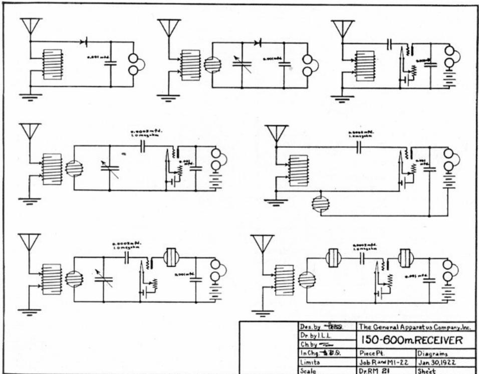
Fig. 1. Some of the many circuits in which the variocoupler can be employed
