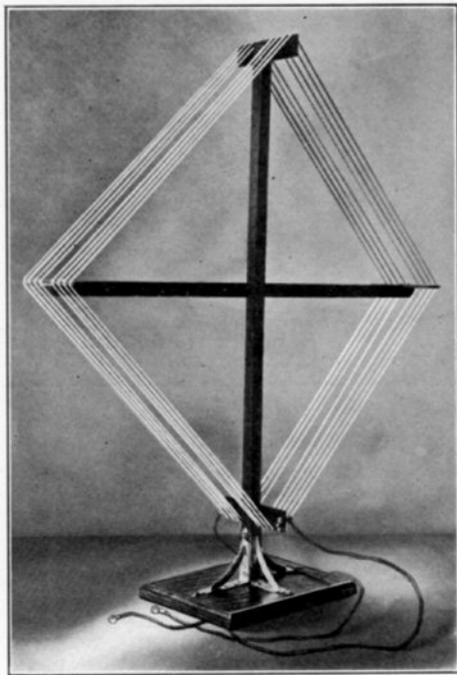
Fig. 6. The loop Antenna
