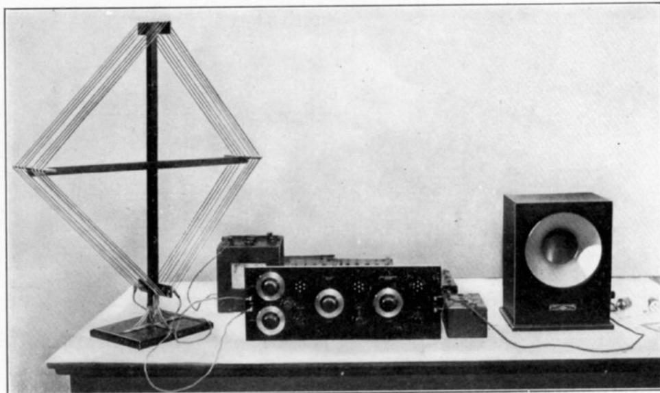
Fig. 8. Complete super-regenerative receiving equipment
