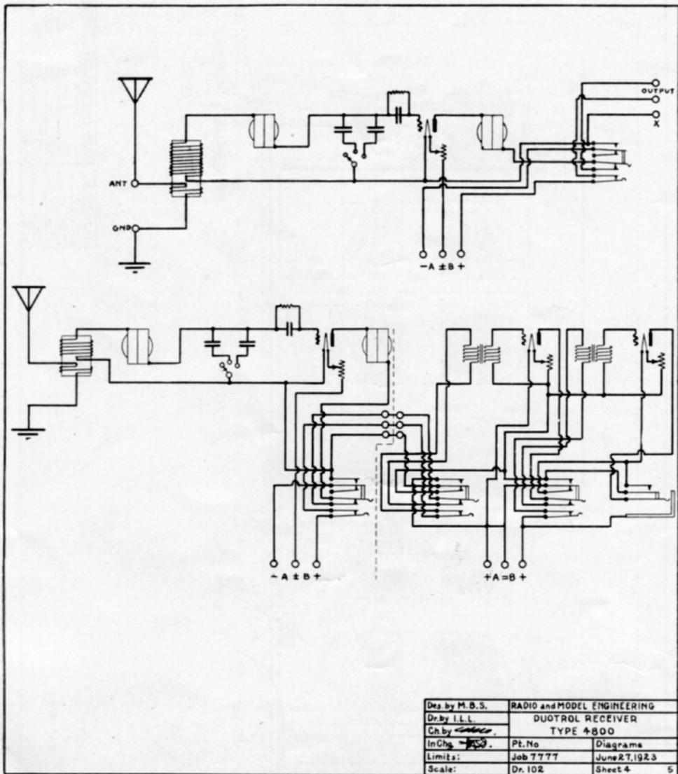
Fig. 9. A schematic diagram of the set, and below a complete diagram of the set and a separate filament control amplifier
