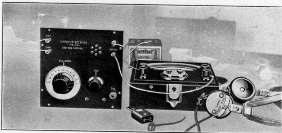
Fig. 1. The set as it was hooked up for measuring the plate current of the W. T. 501 tube. A Rawson micro-ammeter was used to indicate the current
