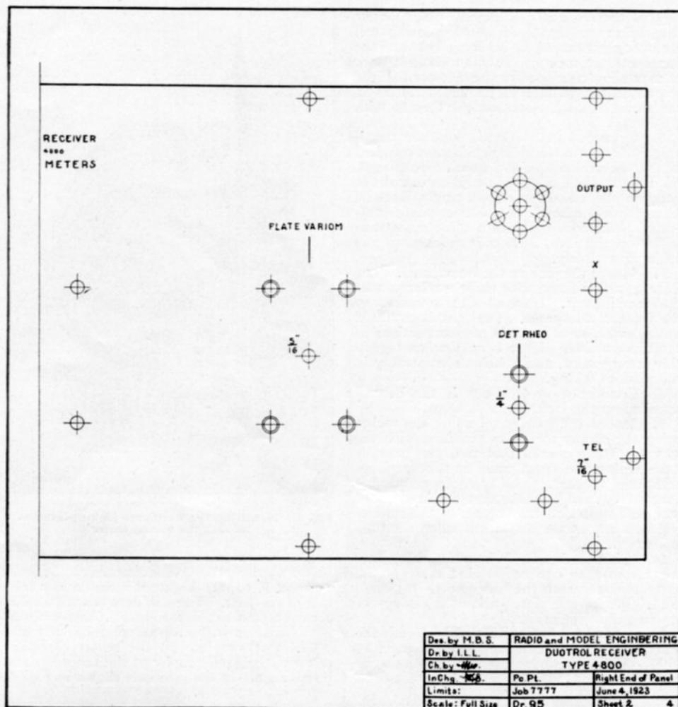
Fig. 6. The right hand half of the front panel, at one-half scale. Concentric circles indicate countersinking for flat head screws
