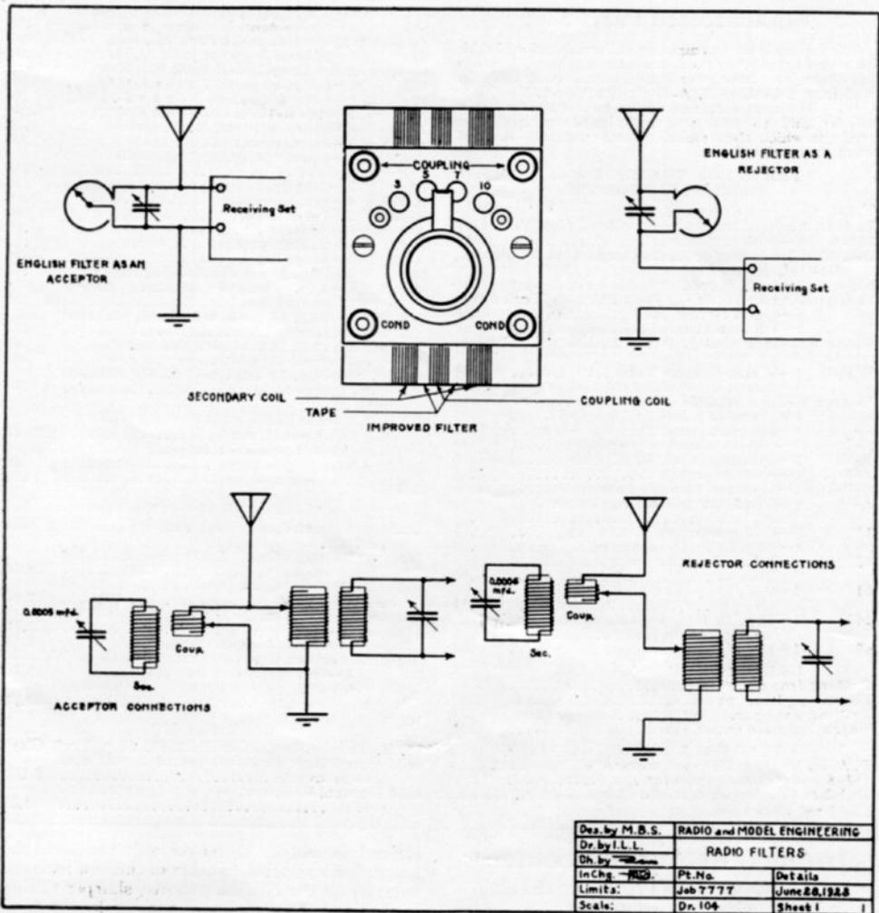
Top, left, the English acceptor connected across the antenna and ground posts of a receiving set. Right, the rejector similarly connected. Center, the assembled improved filter, ready for use. Below, left, a new type filter used as an acceptor. Right, the filter as a rejector. Similar connections can be used for any type of receiving set
