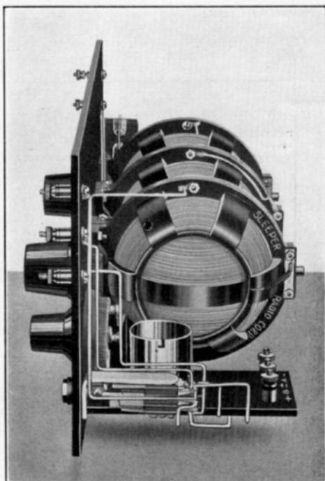
Fig. 4. Mounting the telephone jack upside down makes the wiring easier
