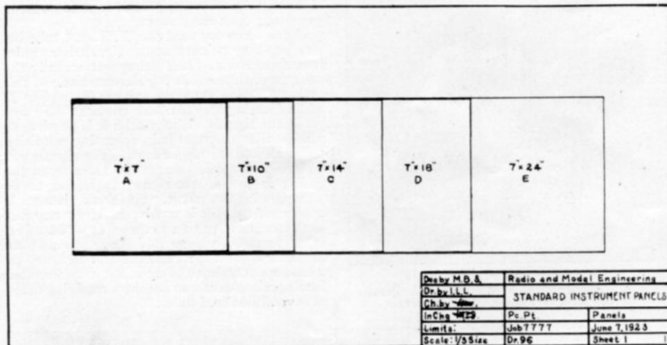
Fig. 1. One-sixth scale drawing of standard instrument panels used for receiving sets
