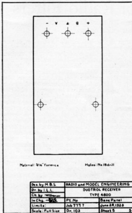
Fig. 7. One-half scale drawing of the base panel, showing the location of the holes
