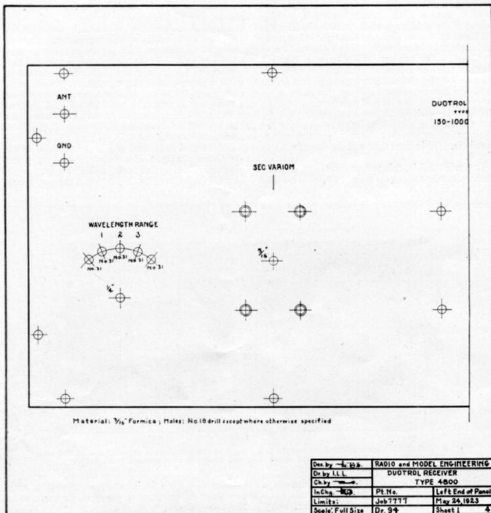
Fig. 5. Because of the extra length of this panel, the drawing was divided into two parts. This shows the left hand half at one-half scale
