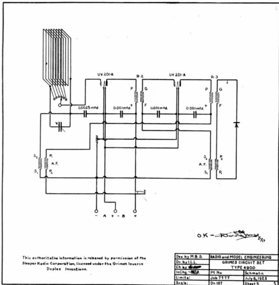
Fig. 9. Schematic diagram showing the arrangement of the Inverse Duplex Circuit
