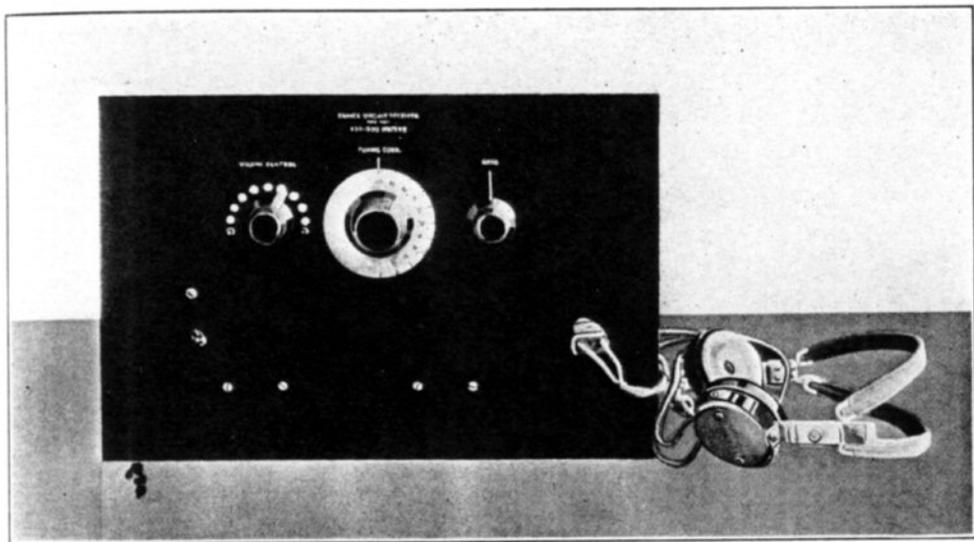
Fig. 1. The set ready to operate. Since the loop can be mounted directly behind the panel this makes a most convenient table unit
