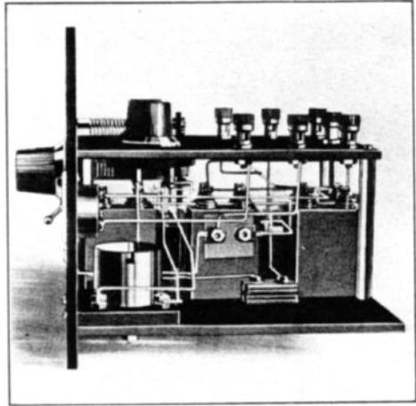
Fig. 5. Here the three audio transformers and the 0.005 mfd. condenser can be seen
