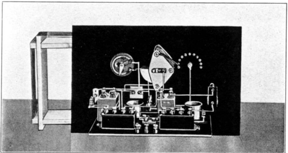
Fig. 2. The loop, shown at the left, fits right around the instruments which are mounted at the rear of the front panel
