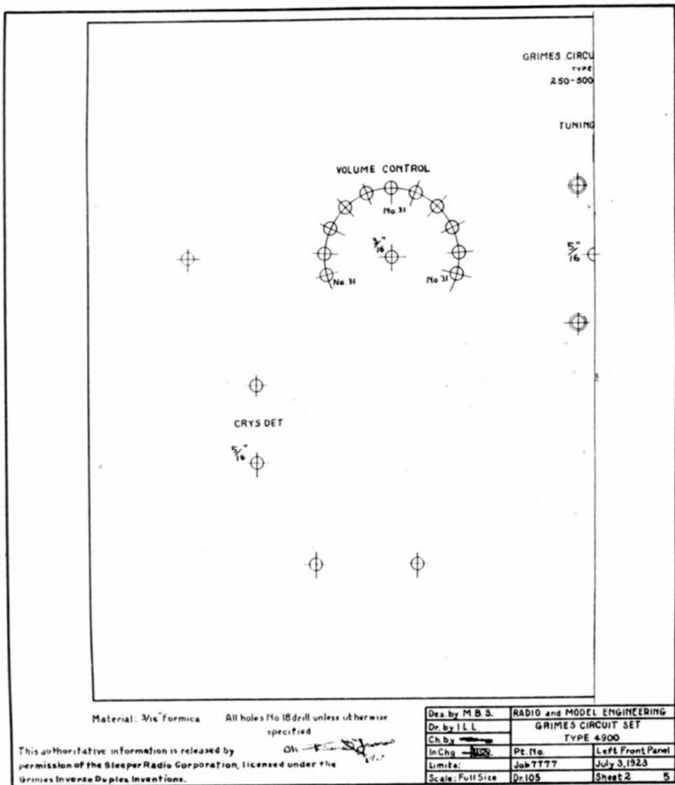
Fig. 5. A one-half scale drawing of the left-hand half of the front panel
