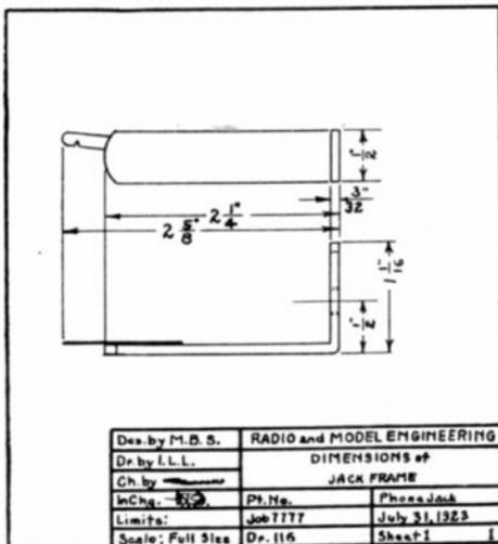
Fig. 8—Phone jack details at one-half scale
