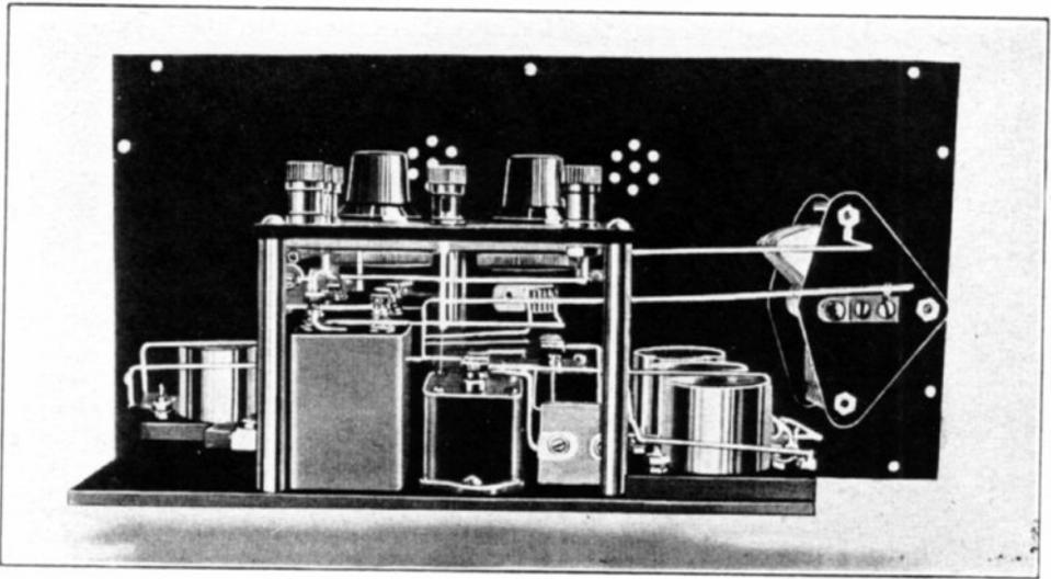
Fig. 4. In the rear view you can see the arrangement of the base and the terminal panel, supported on three pillars
