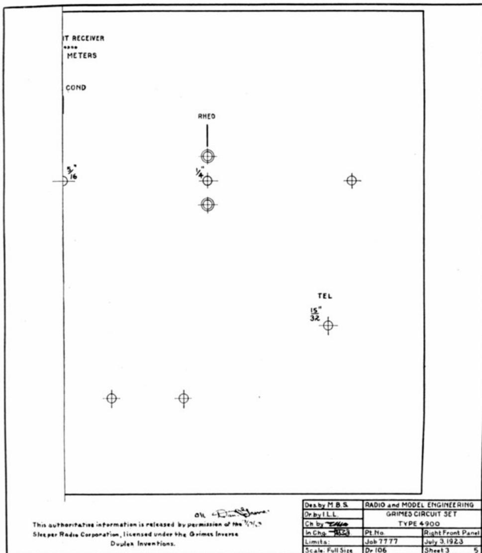
Fig. 6. The right-hand half of the front panel, one-half size. Concentric circles indicate countersinking
