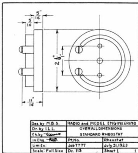
Fig. 5—One-half scale drawing showing standard rheostat features
