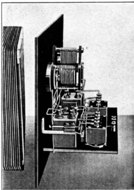
Fig. 3. The set ready for mounting the loop antenna
