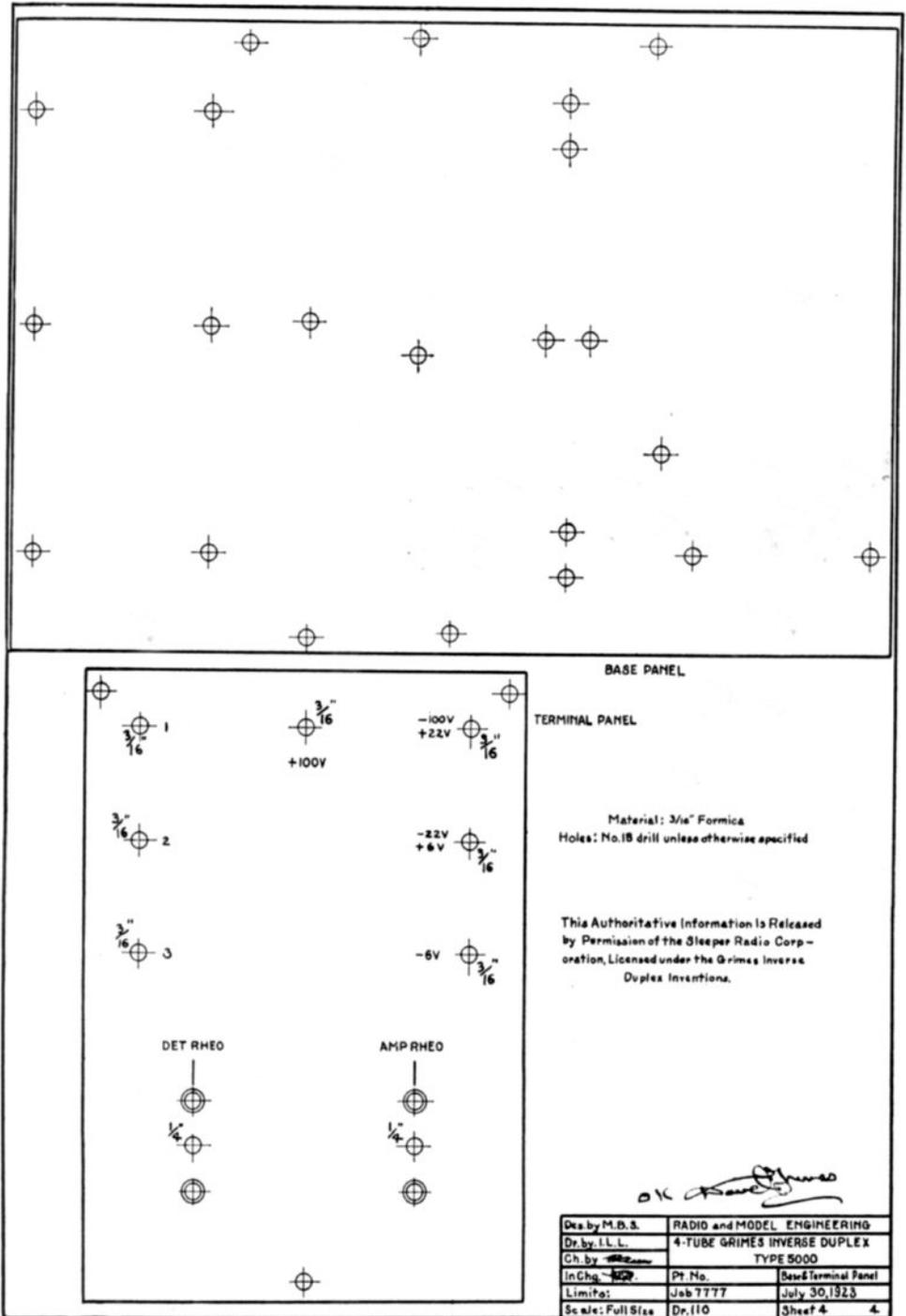
fig. 7. One-half scale drawing of the base and terminal panels. Engraving for the binding posts is also indicated
