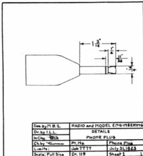
Fig. 7—One-half size drawing of the phone plug
