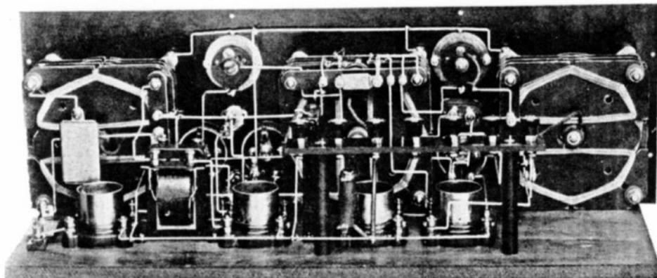
Rear view of the outfit removed from the cabinet. Note the construction of the D coil variable transformers
