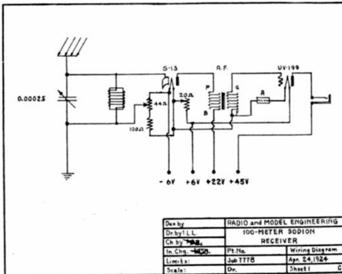
Fig. 2. Wiring diagram of the Sodion set for 100-meter reception
