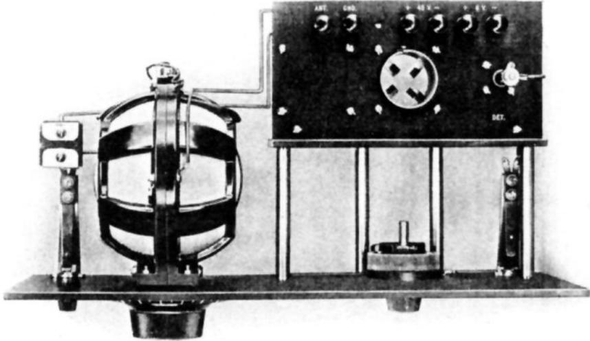
Fig. 2. Only two wires running to the tube panel are required. The rest of the connections are supplied by the panel supports
