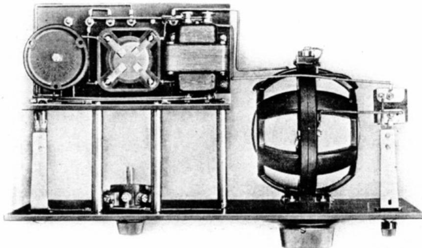
Fig. 6. Looking underneath at the works of the set. You can see the R. F. transformer, socket, and A. F. transformer
