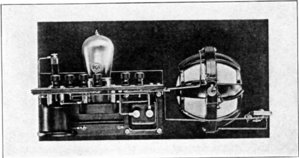
Fig. 1. The fixed crystal, mounted at the left of the tube, can be seen, as well as the supporting arrangement for the socket
