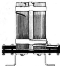
The only way to an inductance more efficient than the Single Layer Coil on a tube is to remove the tube—to remove the dielectric absorption. The Bureau of Standards winds coils on frames. PICKLE BOTTLE COILS are ENTIRELY SELF-SUPPORTING.
