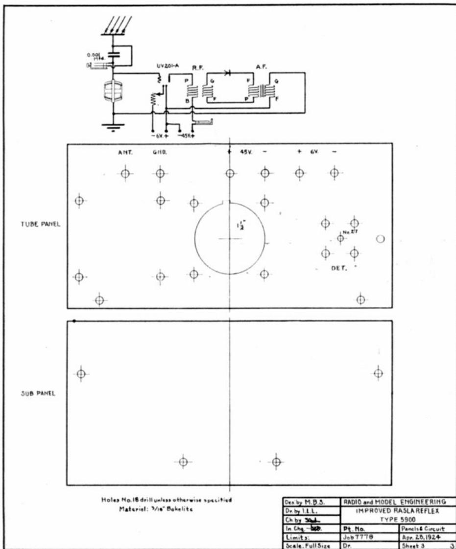
Fig. 4. Schematic wiring diagram and one-half scale drawings of the tube and sub-panels
