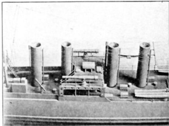
Fig. 7. Looking down amidships on the port side. The superstructure, with the 4-in. R. F. guns and fittings, is clearly shown, as well as the arrangement of the deck. At left is the ladder from the oridge, views of which have been given already. Such details as are hidden under the superstructure will be illustrated subsequently
