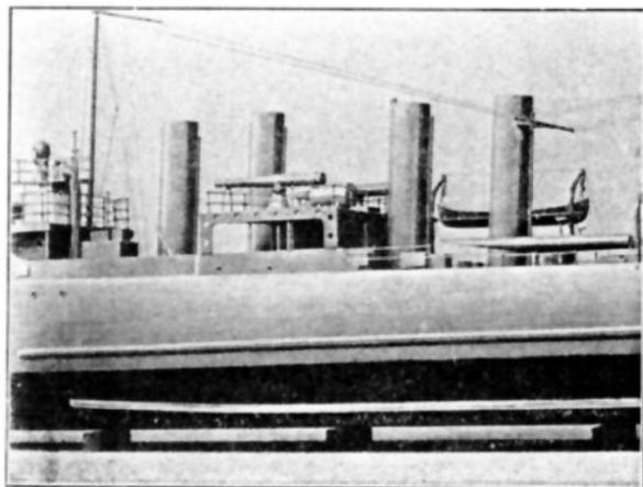
Fig. 9. Here the bridge shows more plainly. The tall ventilator is made by mounting an ordinary short ventilator on a wooden dowel. The life boat and the torpedo tubes are illustrated also. Port holes can be turned out of brass tubing, or they can be purchased either plain or fitted with glass
