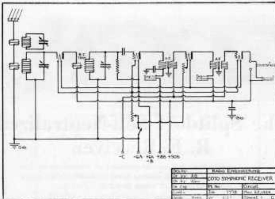
Fig. 2. Schematic wiring diagram of the Coto Symphonic receiver.
