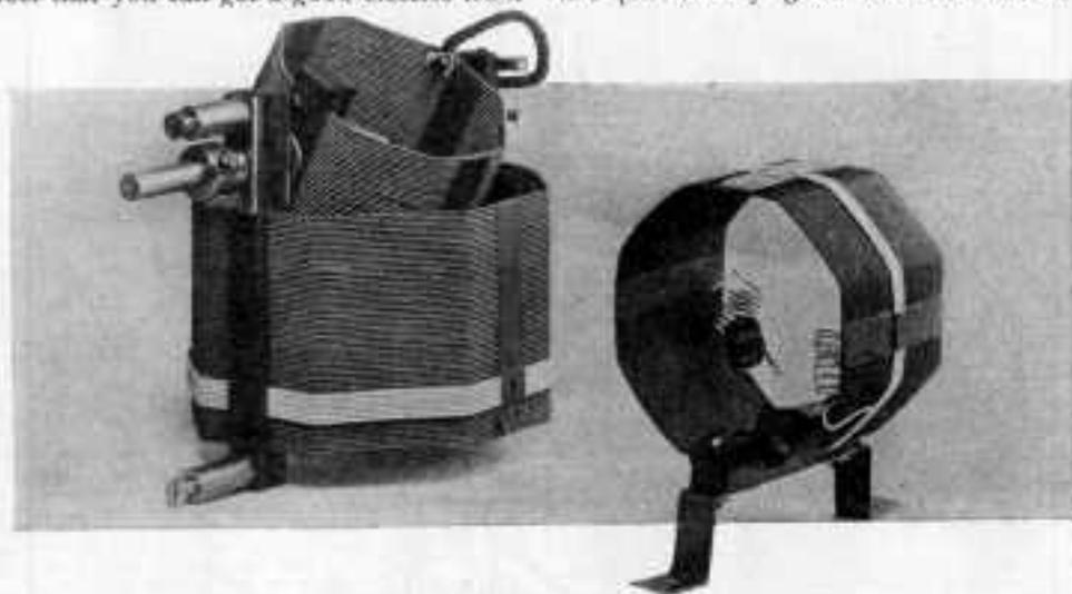
Fig. 5. A close-up of the pickle-bottle type tuner and coupler. The coupler shaft is cut off as it is not needed.
