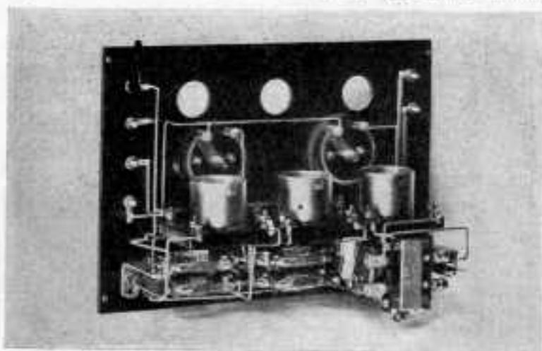
Fig. 2. A rear view showing the mounting of the transformer and resistance units beneath the sockets.
