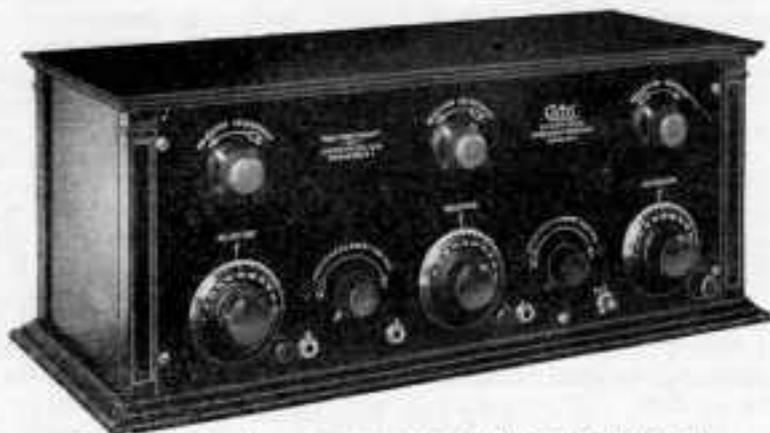
Fig. 3. Showing the arrangement of controls for tuning the set.
