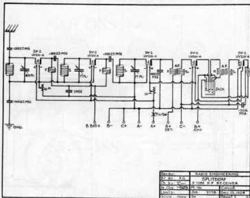
Fig. 2. This wiring diagram shows the circuit system employed for the Splitdorf receiver.
