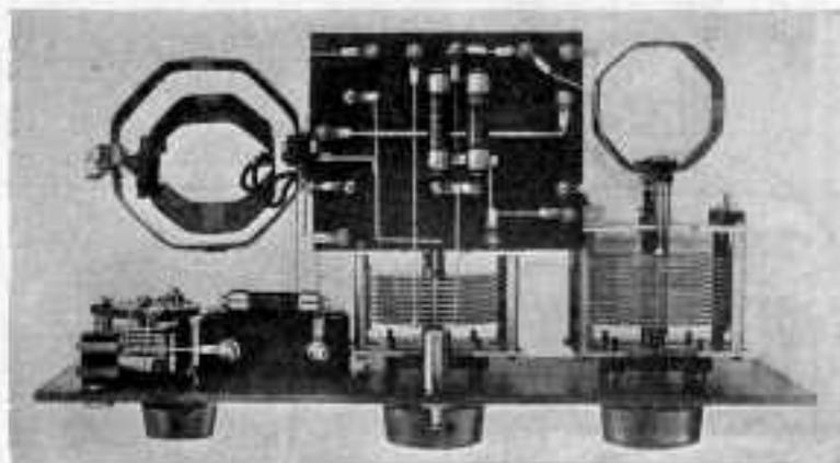
Fig. 6. A bottom view showing the Amperites, R.F. transformer, and fixed crystal detector.
