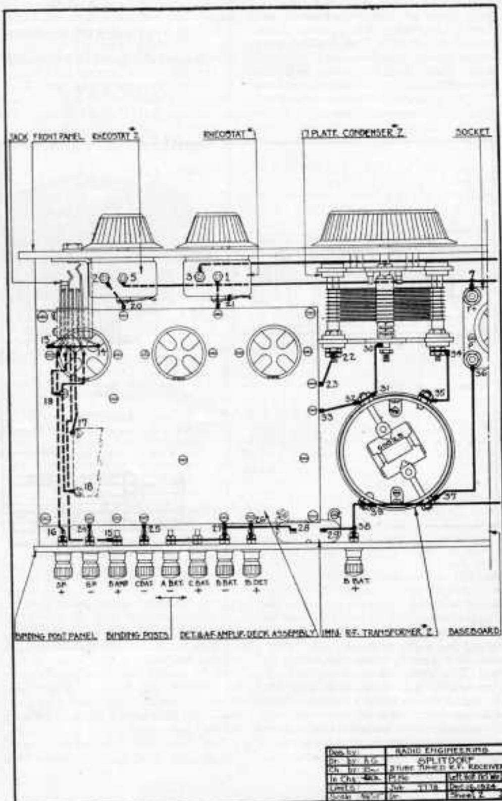
FIG. 2. Picture wiring diagram of the left hand half of the set.
