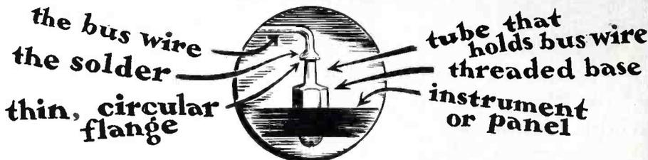
The Standard, tubular Soldering Terminal
