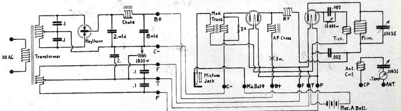
Fig. 2. Connections for the power supply, at the left, to the US-76 short wave telephone transmitter, at the right
