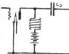
Fig. 8. The value of  $C_3$  determines the amount of regeneration in the plate circuit
