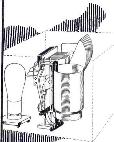
*Automatic Variable Coupling*—same control operates tuning condenser and primary coil coupling simultaneously, gives maximum and equal amplification and selectivity over entire tuning range.
