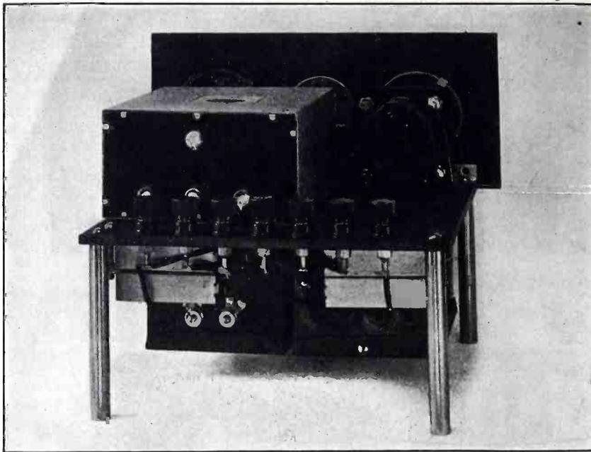
Fig. 1. Rear of the US-76 eliminator. Note that the Raytheon tube is mounted horizontally
