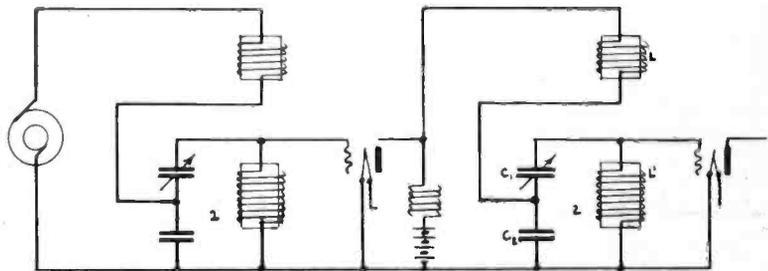
Fig. 7. Complete circuit of the Loftin-White receiver. This is one of the applications of the system. Using this method, it is possible to obtain a sufficiently constant regeneration to make a single-control, 3-circuit tuner
