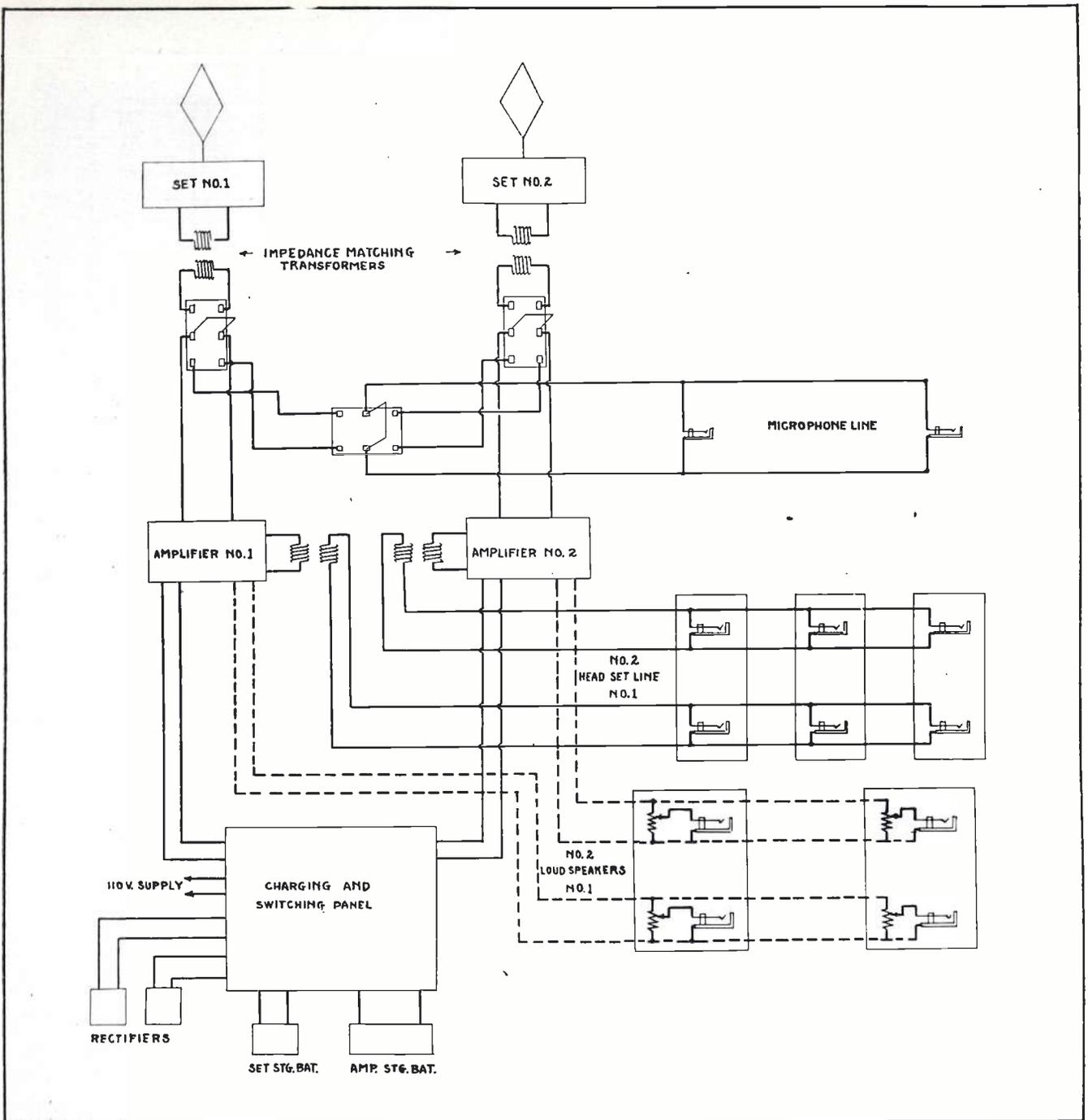
Fig. 1. Schematic diagram of the Western Electric installation at the Sydenham Hospital, in New York City
