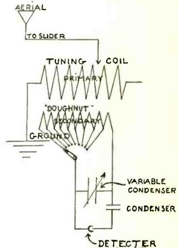
Fig. 29. Wiring arrangement of a radio receiving circuit employing a "doughnut" tuner. The transmitting telephones were connected in shunt with the detector.
