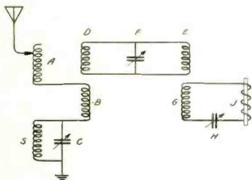
Fig. 37. Circuit diagram of the Marconi multiple tuner.
