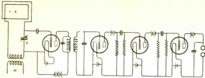
Fig. 41. General circuit of early Superheterodyne receiver.
