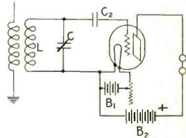
Fig. 34. Circuit employing the three-electrode audion—patent issued to deForest, February 18, 1908.
