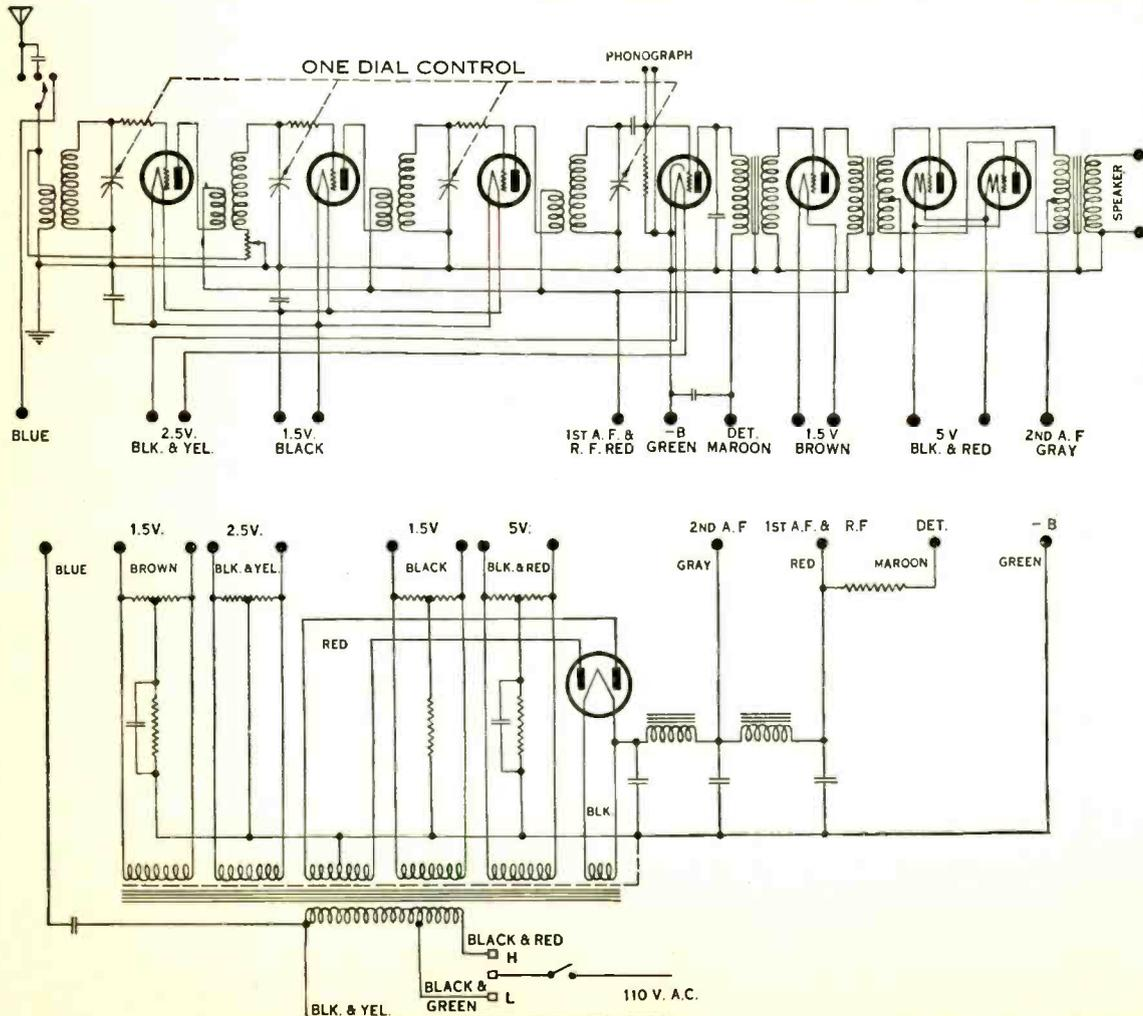
Schematic diagram of the Stewart-Warner Model 801-A, Series B, a-c. receiver.
