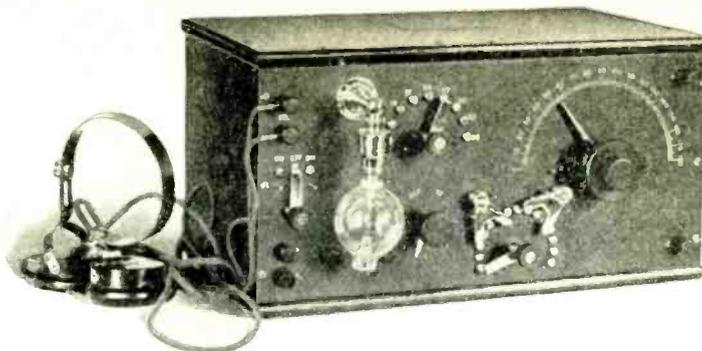
Fig. 36. Radio receiver of the year 1913, comprising an audion detector and contained tuning element with "dead end" switches.
