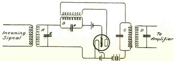
Fig. 42. Circuit arrangement of second-harmonic superheterodyne.
