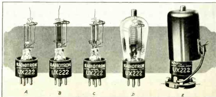
The intricate construction of the UX-222, let alone all a-c. tubes, suggests the difficulties encountered in manufacture when automatic machines replace hand work.
