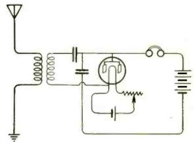
Fig. 33. Typical audion receiving circuit of 1906.
