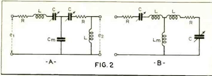
Two generalized band-pass filter circuits. The inductances L, in Fig. 2-B should be indicated as  $L_1$ .
