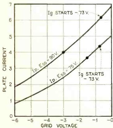
Comparative curves of screen-grid tube with old and new rating.
