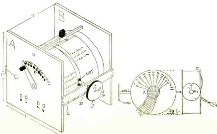
Fig. 28. "Doughnut" receiving tuner of the period around 1910. A, and B, are the retaining ends; F, the secondary contact switch; D, adjusting shaft, and J, a handle by means of which the coupling is varied between primary and secondary.
