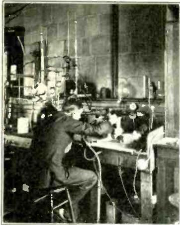
An authority on gaseous rectifiers studying the glowing tube in order to determine, by means of the spectrum, the chemicals present.
