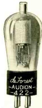
The new DeForest "422 D.C." screen-grid tube, which has a heavy oxide-coated filament.
