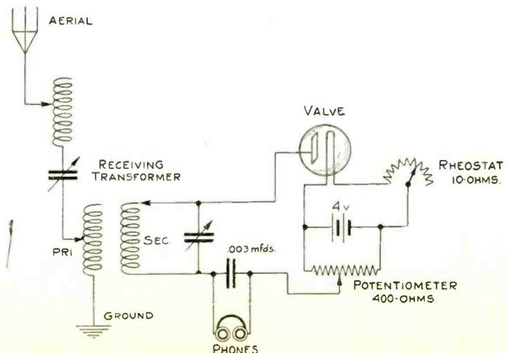
Fig. 32. Receiving circuit employing the Fleming valve detector.
