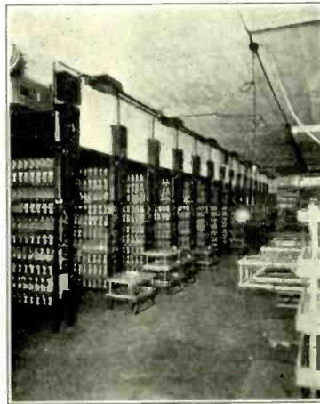
From these life racks the tube manufacturer can learn just what he can expect of the tubes in actual use. This is the production testing feature of engineering.
