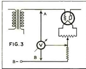
Manner of making grid voltage test.
