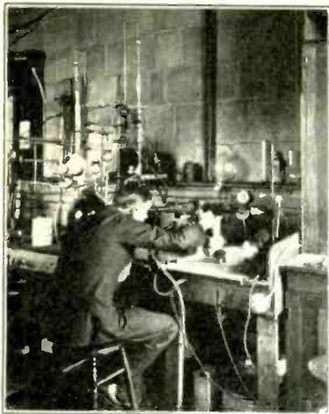
An authority on gaseous rectifiers studying the glowing tube in order to determine, by means of the spectrum, the chemicals present.
