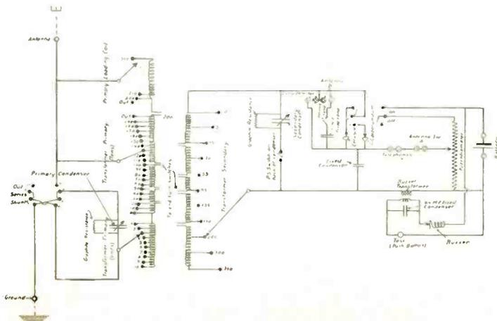
Fig. 35. Schematic diagram of the Marconi Receiver of 1913.
