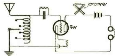
Fig. 39. Schematic diagram of early single-circuit regenerative receiver.
