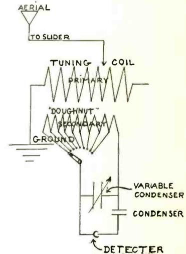
Fig. 29. Wiring arrangement of a radio receiving circuit employing a "doughnut" tuner. The transmitting telephones were connected in shunt with the detector.
