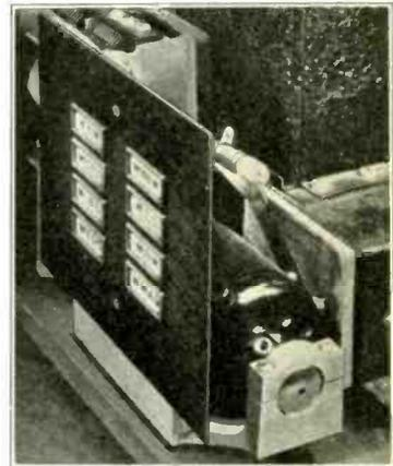
Showing the tab push-buttons and the driving motor of the Carter tuning system.
