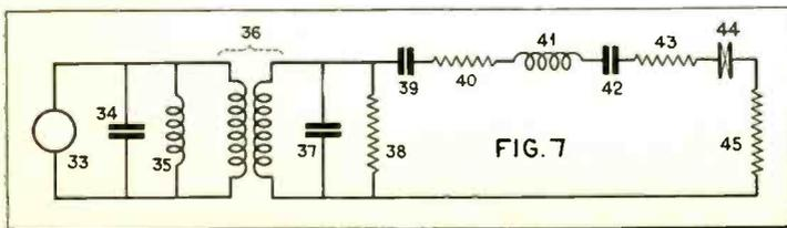
Equivalent circuit diagram of magnetic pickup shown in Figs. 1 and 2, in Part I of this article.
