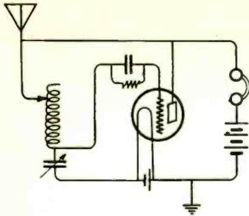
Fig. 38. The Ultra-audion circuit of 1913.
