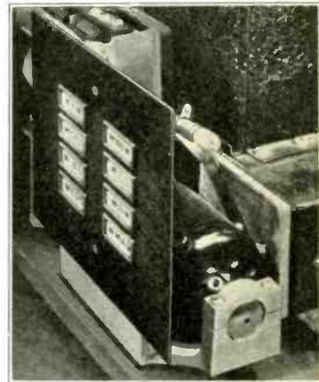
Showing the tab push-buttons and the driving motor of the Carter tuning system.
