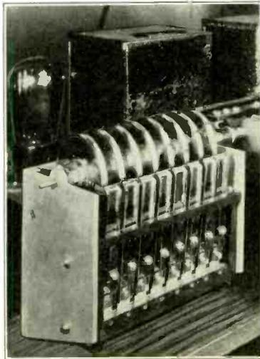
The station selector mechanism of the new Carter remote tuning control system.
