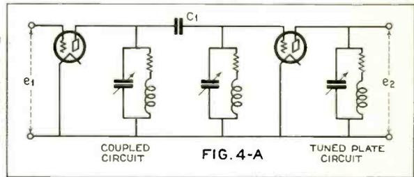
Since ordinary tuned circuits are broader at the high frequencies, a stage of capacitive coupled tuned circuits will tend to offset this tendency. Of course R has to be small enough to make
