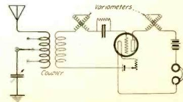
Fig. 40. Two diagrams of early two-circuit regenerative receivers.
