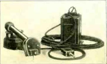
Stromberg-Carlson electric pickup for power detector circuits.
