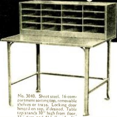
No. 3040. Sheet steel. 16-compartment sorting top, removable shelves or trays. Locking door hinged on top, if desired. Table top stands 30" high from floor, 33" deep and 41 1/2" wide, 16-gauge sheet steel. Legs, 1 1/2" angle steel. Finish, olive green enamel.
