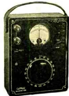
All DayRad Instruments are equipped with genuine D'Arsonval movement meters.
