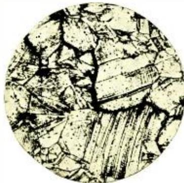
Fig. 1. In this photomicrograph it may be seen how the crack follows the crystal boundaries.
