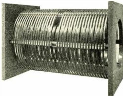
We make to individual order inductances for tank, antenna tuning and similar circuits. Sturdy wood frames, special shaped one-piece conductors and Isolantite insulators. No metal other than the conductor used in construction. Tank Condensers also built to order.
