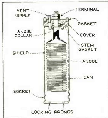
Fig. 1. Construction of the Electrolytic Condenser
