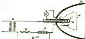
sound reproducers in which a continuous corona discharge is provided, the discharge being modulated by a sound modulated current such as is obtained from a radio receiver.
