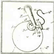
of the invention is to provide a new and improved tuning arm to which a telephone receiver may be attached above the top board of the phonograph without removal of the phonograph sound box and independently thereof.
