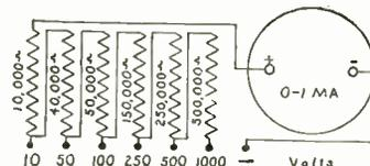
**Bulletin 100-M** completely describes with many charts and diagrams the many uses for Super Akra-Ohm Resistors. Send for your copy today. Let us know your resistor specifications and we will quote you on the proper type required for your work.
