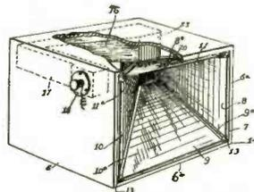
and it is the object of the invention to provide a sound amplifier of this character, which is novel, compact and cheap in structure, and highly efficient in propagating and magnifying the sound waves of dominant and undertones.
