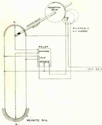
Fig. 1. Schematic of remote tuning circuit.
