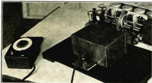
Fig. 3. Remote tuning system as applied experimentally to a Philco Model 95 chassis. Tuning unit shown at left.
