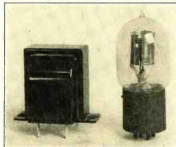
A radio transformer compared to ordinary radio tube.
