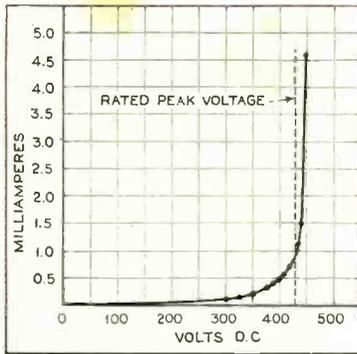
Fig. 2. Variation of leakage current with voltage.
