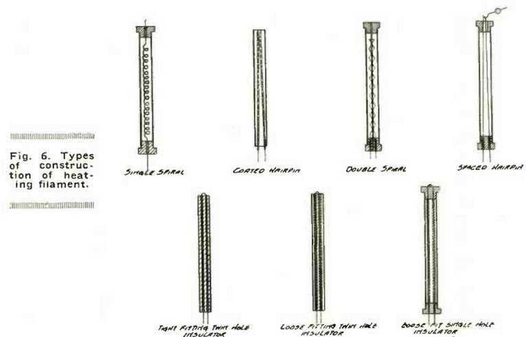
Fig. 6. Types of construction of heating filament.
