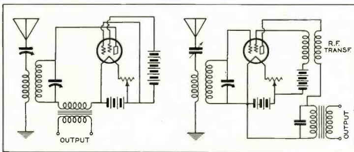
Fig. 5. This circuit shows the action of the tube as a rectifier. This circuit combined with that of Fig. 6, make the complete layout of Fig. 7.
