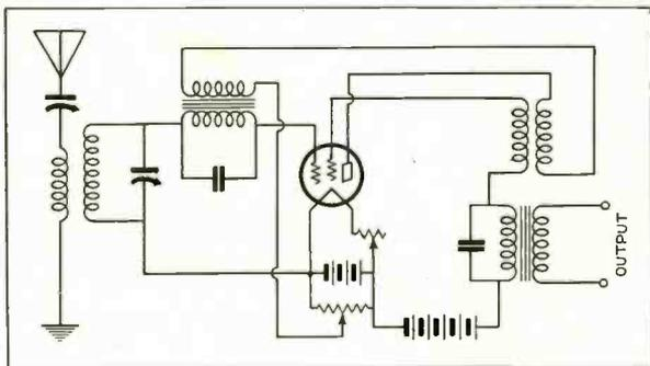
Fig. 7. Complete circuit capable of radio-frequency amplification, detection and audio amplification, with but one tube.
