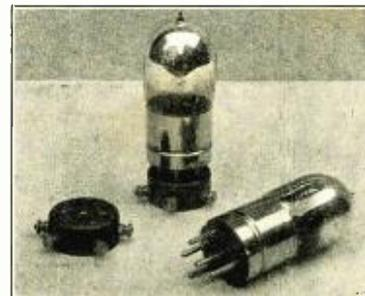
Fig. 2. Foreign double-grid tubes. Note base construction and special sockets.
