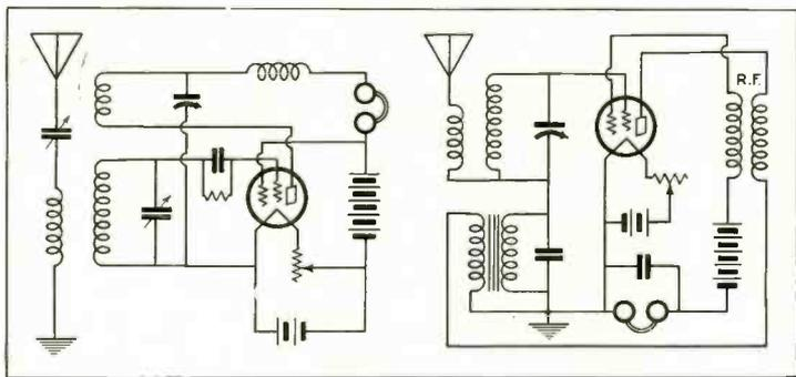
Fig. 3. Short-wave double-grid tube circuit.
