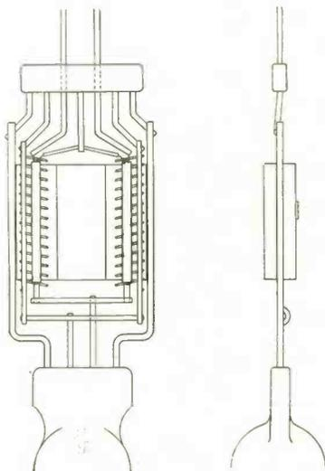
Fig. 1. Early 5-volt heater tube assembly.
