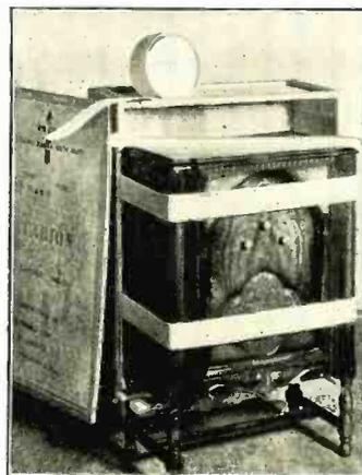
*Clarion Radio, manufactured by Transformer Corp. of America. Strips of Ribbon KIMPAK distribute the packing pressure evenly over the greatest possible bearing surface.*
