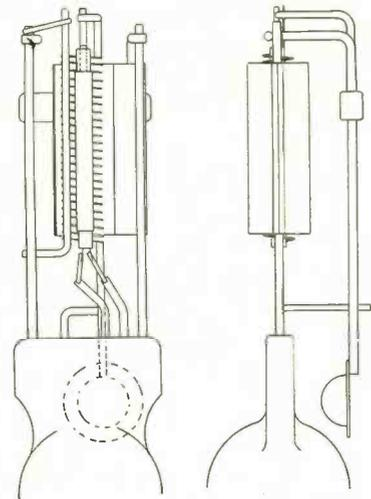
Fig. 2. Heater type tube assembly, for automatic manufacture.
