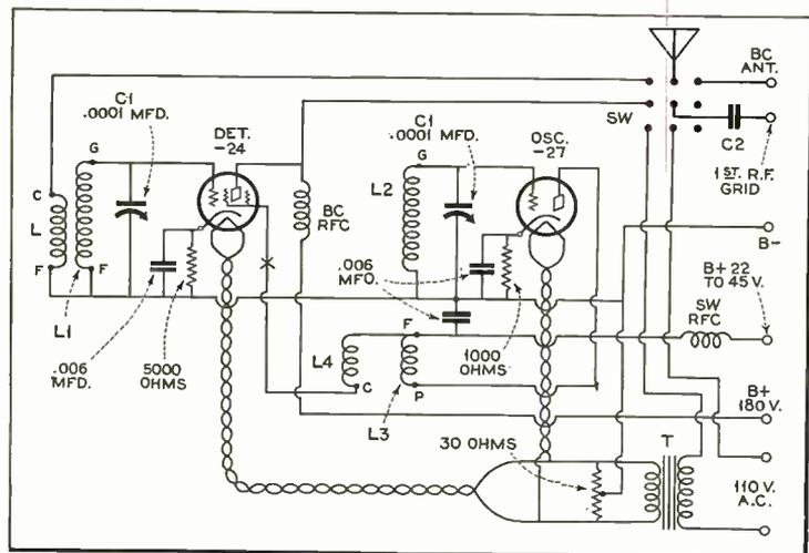
Fig. 1. Circuits of Tanner converter.
