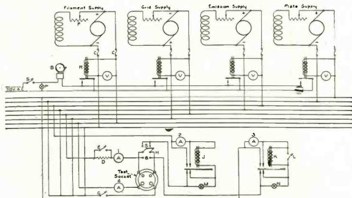
Fig. 1. Wiring layout of test panel for production testing of tubes.
