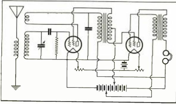
Fig. 15. Two-tube receiver the equivalent of three stages of audio amplification.
