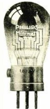
Fig. 1. Multi-grid tube.
