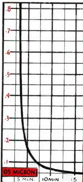
The CENCO HYPERVAC PUMP is very small relative to its large capacity. It exhausts so low that a guarantee of 0.05 microns can be given—*20 times better than any previously guaranteed vacuum . . . the first pump of its kind to combine large volume displacement with the ability to reach exceedingly low pressures.* This combination speeds up the production of high vacuum in a system (see chart at left). Power requirements low. For further information address us at 460 East Ohio Street, Chicago.
