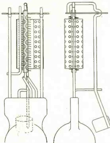
Fig. 8. Construction of perfected quick-heater audion.
