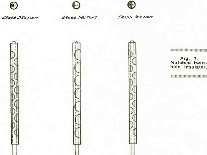
Fig. 7. Notched twin-hole insulator.
