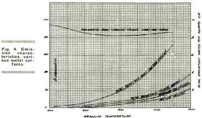
Fig. 4. Emission characteristics. Various metal surfaces.
