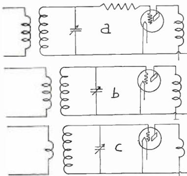
(c) Stabilizing by putting very few turns on the primary coils. This keeps the inductance in the plate circuit below that required to make the tube oscillate.
