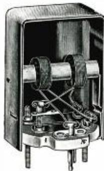
soldering. The coils are wound with No. 36 SSE wire of special type insulation to provide maximum inductance and low distributed capacity.
