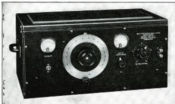
This beat-frequency oscillator is a new development in sources of audio-frequency voltage for test purposes. It covers a wide range (5 to 10,000 cycles per second) and its waveform is excellent. Accurately calibrated.
