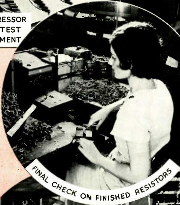
FINAL CHECK ON FINISHED RESISTORS
