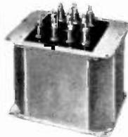
*UTC Transmitter Components* are used by discriminating commercial organizations and experimentors to obtain superior, long lasting results. The unit illustrated is an output transformer designed to match Class B 203's or A Prime 845's to a 6,500, 5,000 or 3,500 ohm load.
