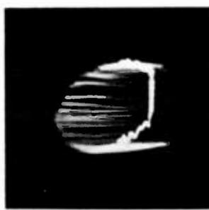
Fig. 57. Composite wave of 60-cycle pickup and commutator ripple.
