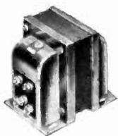
A typical value in the new **CHROMSHIELD FILAMENT TRANSFORMERS**, outer shields chromium plated—bakelite terminal strips—with new type solder or screw terminals. Will handle 4-83's in bridge rectifier circuit, insulated for 5,000 volts.
