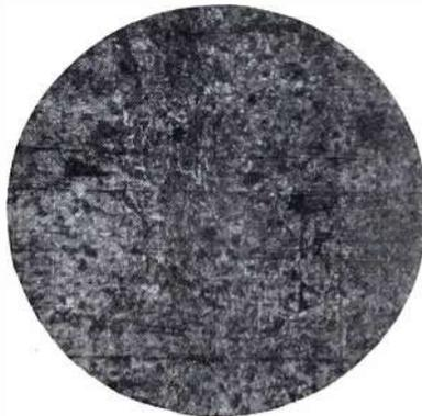
Flat strip of nickel for radio: Surface with no polishing or etching (100X unretouched). Note relative porosity and non-uniformity of surface.
