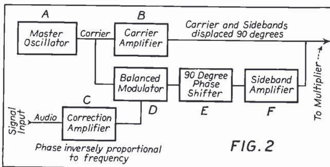
Block schematic of the essentials for attaining frequency modulation.
