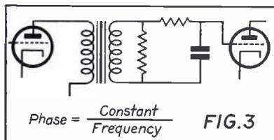
Circuit of the correction amplifier used in the frequency modulation system.
