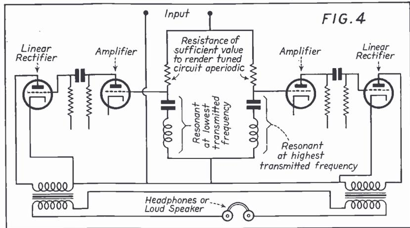
Circuit used in the receiver for converting frequency modulation to amplitude modulation.
