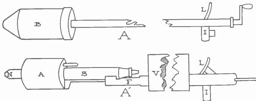
Fig. 3. (A') By pulling the lever L the intake I and the nozzle N open, as the section S moves back and forth on F. The chamber A contains the binder material, while V is a vacuum space. (A) By opening the valve by means of L and rotating the crank slowly, the fluorescent powders in B are forced out by the pressure of  $\frac{1}{2}$  to  $\frac{3}{4}$  atmospheres. Overall length of guns, 12 inches. (Courtesy of Pfaltz & Bauer.)
