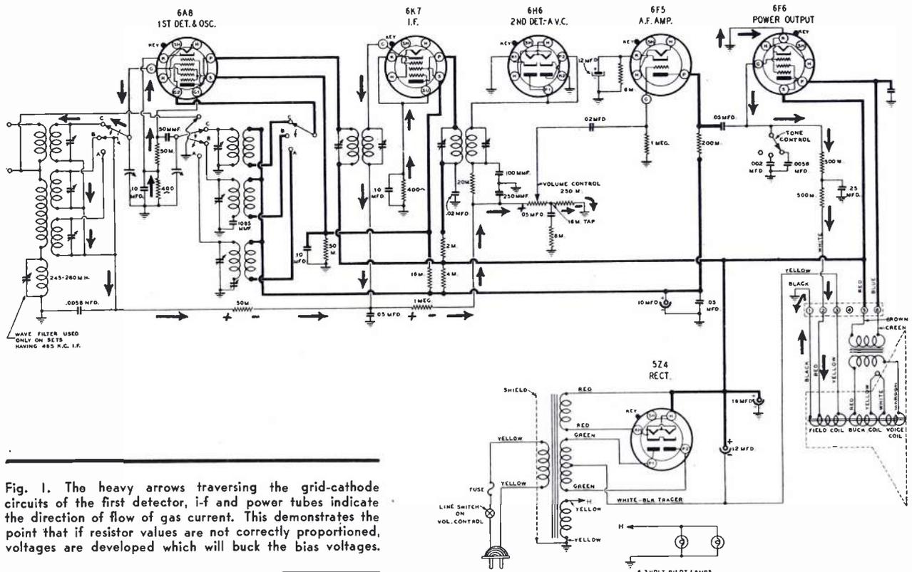
Fig. 1. The heavy arrows traversing the grid-cathode circuits of the first detector, i-f and power tubes indicate the direction of flow of gas current. This demonstrates the point that if resistor values are not correctly proportioned, voltages are developed which will buck the bias voltages.
