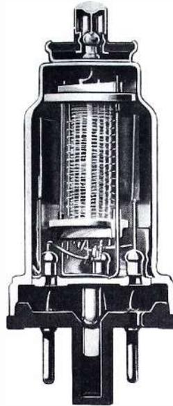
(Courtesy Raytheon Production Corp.) Interior structure of representative metal tube, cut away to show the positions of the elements.
