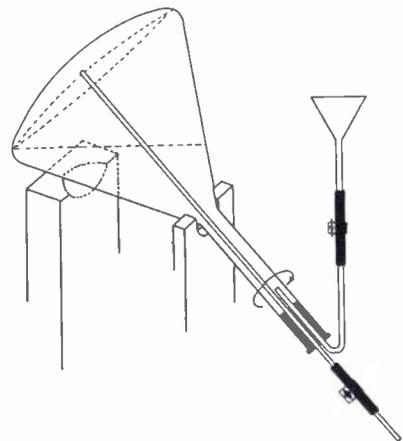
Fig. 1. Funnel method, as employed in this country on both an experimental and small-production scale, for coating the interior walls of cathode-ray tubes.
