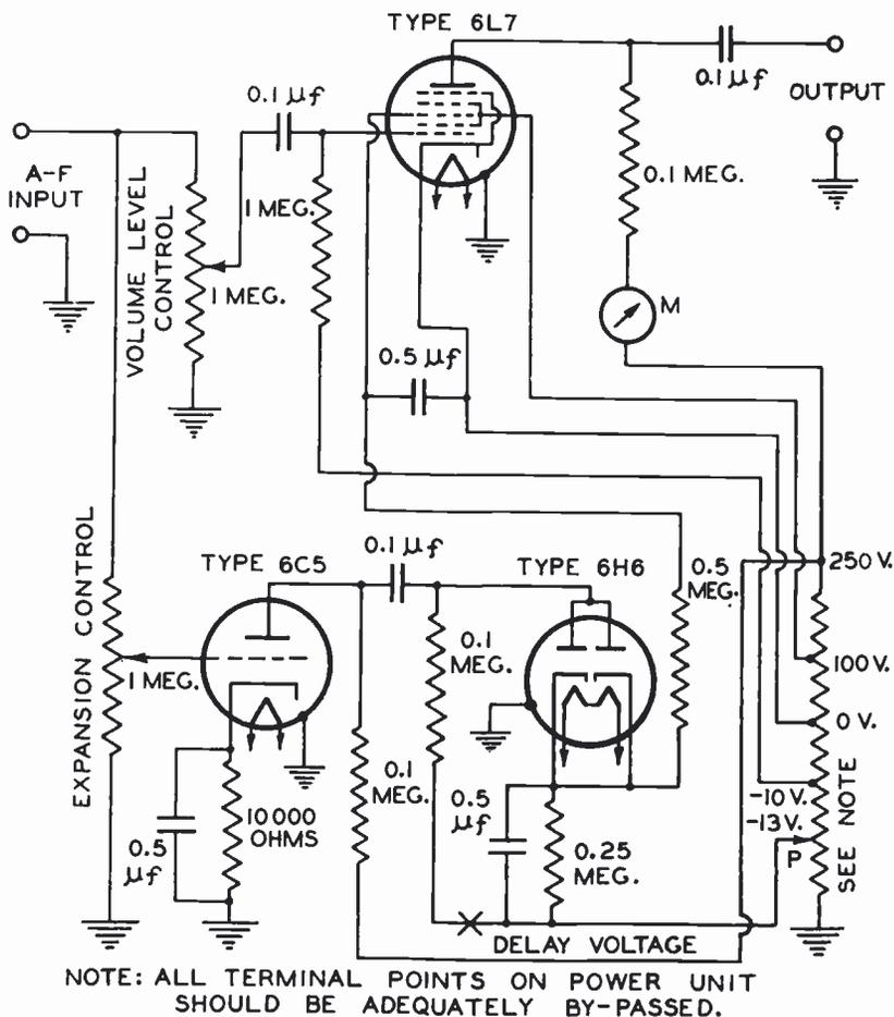
Fig. 1. Volume-expander circuit using a 6L7 tube.
