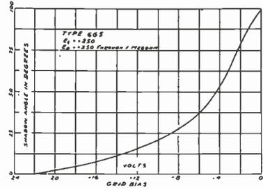
Shadow Angle-Grid Voltage Curve of 6G5.
