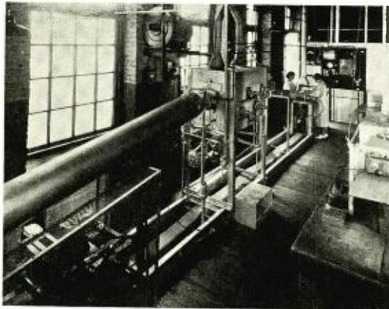
Fig. 3. Hydrogen atmosphere furnaces for brazing metal tubes.
