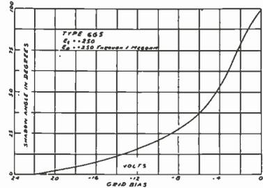
Shadow Angle-Grid Voltage Curve of 6G5.
