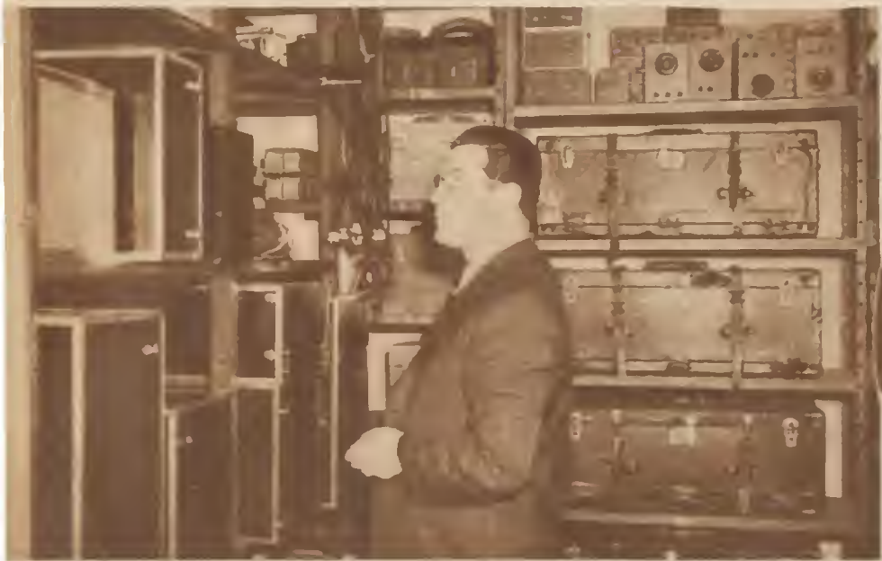
Above: Max Jacobson, head of NBC's Field Division, looks over his equipment. Those portable transmitters (in front of him) are complete broadcasting stations—worth about $2,500 each. The things that look like suitcases are receivers—worth $400 each. With these, two-way communication is possible
