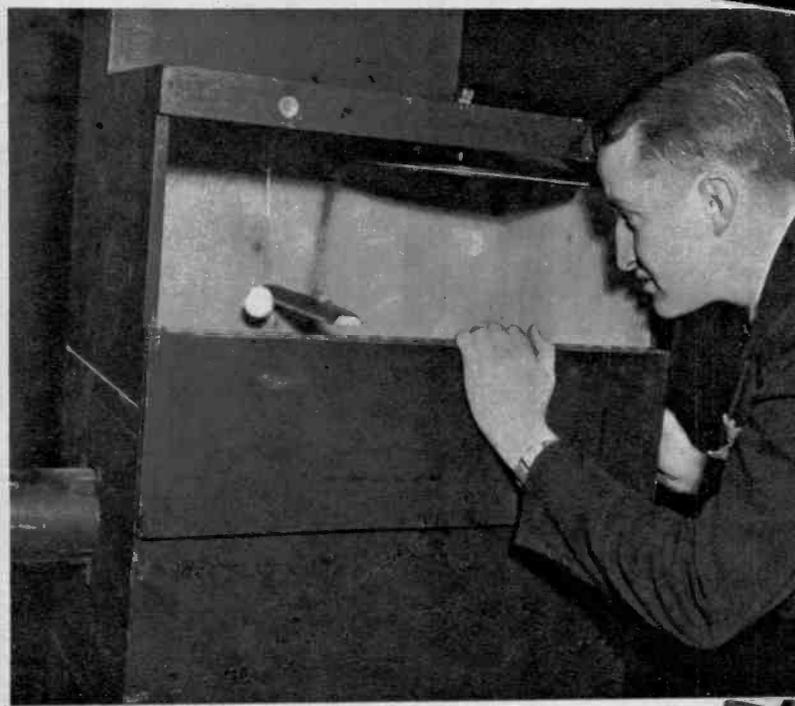
Ray Kelly takes a look into his rain machine. Above the box is a hopper filled with bird-seed. The seed drops down onto the disk, which can be seen on a level with Kelly's head. A wind-shield wiper brushes it off to fall on a triangular shaped board which scatters it. The seed then falls onto several surfaces of different height, rattles on the ping-pong ball!
