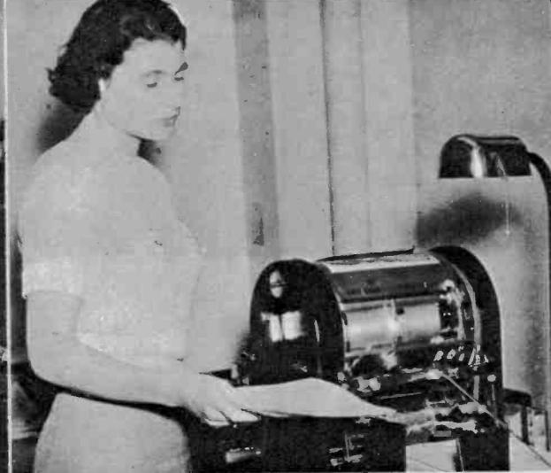
**12** After the prints are developed, and "fixed" in hypo, Dick Schroeder dries them on cloth by heat & air in this machine
