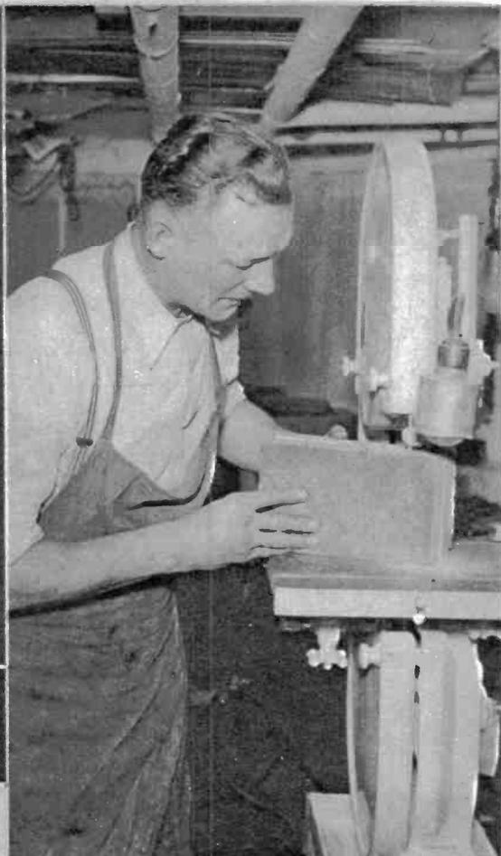
3 The pattern is traced on a block of kiln-dried, 4-ply basswood, and the outline is cut out on a band-saw
