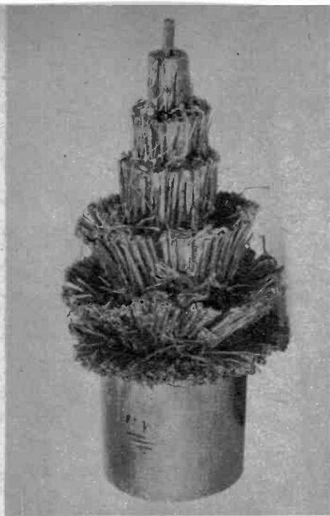
**7** Over 60,000 miles of cable—containing hundreds of wires (above) make up the network
