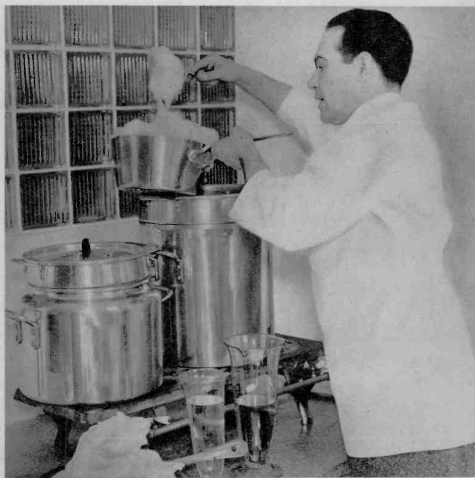
**3** Bagley uses juice from 1 gallon of berries in each 16-lb. batch of cream. Above: Mixing petrolatum (petroleum jelly), lanoline (animal fat), mineral oil and olive oil as base for the cream. He uses no water in any creams
