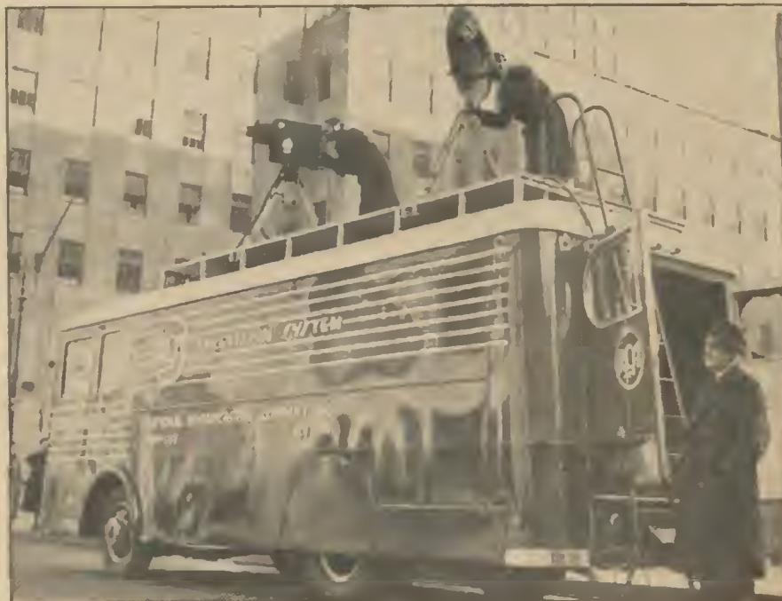
With this first mobile television station, only recently delivered to NBC, the network plans to pick up outdoor events. Note parabolic microphone
