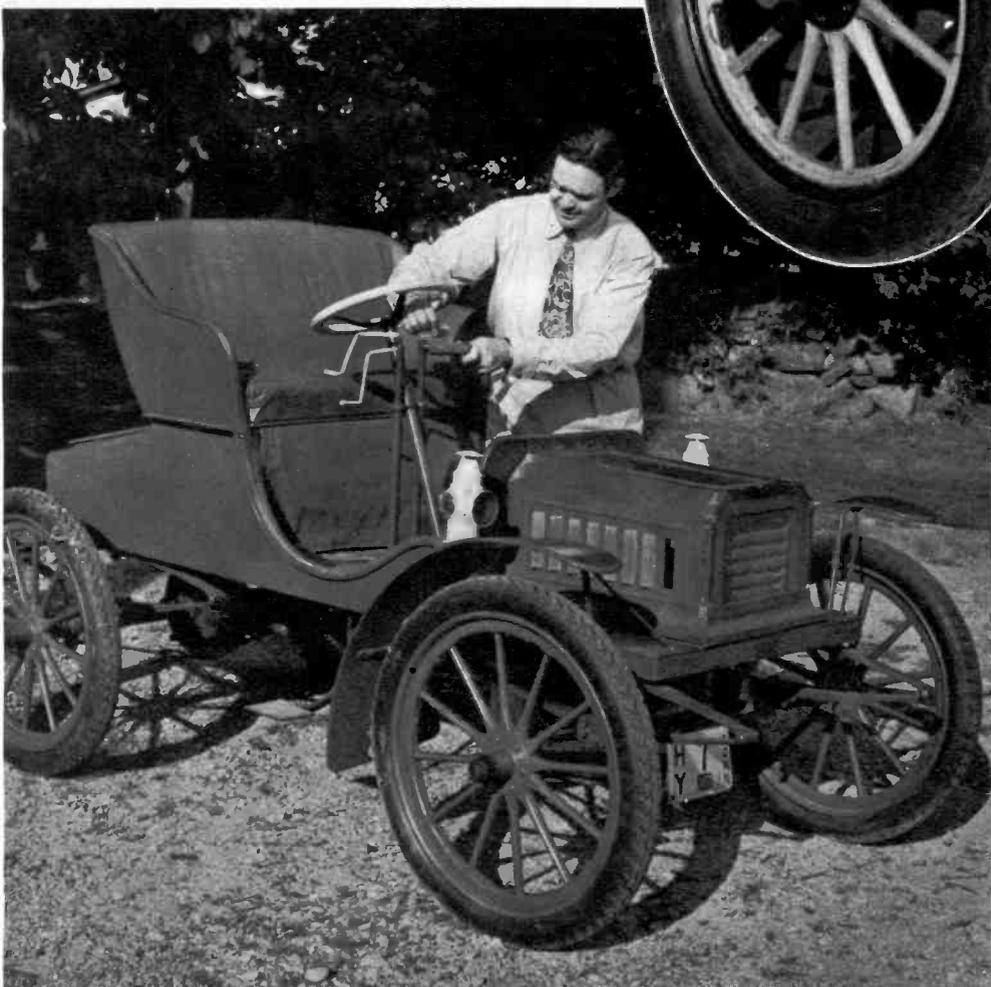
**THE 1904 COVERT-CHAINLESS,** above, just goes to prove that there is nothing new under the sun, for, as Melton points out, the new-fangled gearshift-on-wheel development of today was a part of its make-up
