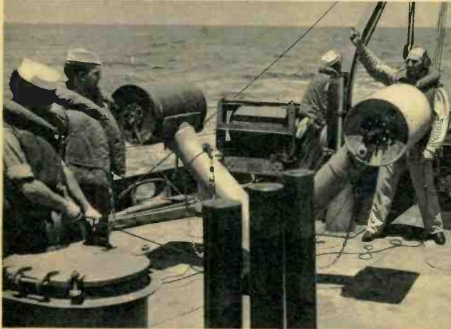
"**READY TO ATTACK!**" A sub's near by, and these Coast Guardsmen have loaded their "Y" gun with two powerful depth-charges. Those harmless-looking drums contain enough explosive to crumple a sub's plates. Sailor at right will pass the fire order
