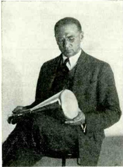
*This bottle-like object is a cathode ray tube which forms the receiver of the new type of television invented by Dr. Zworykin, who is holding it. The broadcast pictures appear on the round end of the tube and from there are projected on a mirror in view of the spectators.*
