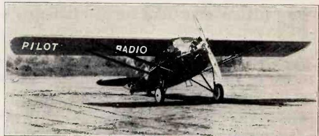
*The plane shown in the picture is a Stinson Detrouter with a J-6 motor which includes a radio cabin, pyralin covered center section for better visibility and a reversible panel in the radio cabin on which a wind driven generator is mounted. When this is swung outward the generator is in use. When swung inward the generator is brought into the cabin, eliminating drag.*
