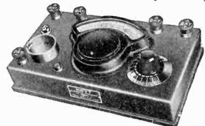
Electrical Instrument Works. By its use all the elements of a tube are tested—filament, grid and plate circuits. Curves can be plotted by the use of a C battery. Voltages of individual cells of A or B batteries can be measured or entire battery voltages measured in blocks of 22 1/2 volts.
