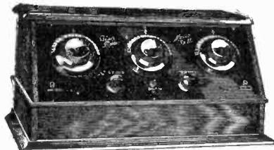
Type—Tuned Radio Frequency (Resistance Coupled Audio); Tubes—6; Battery—"A" Storage or Dry; "B" 135 Volts; Controls—Tuning, 3; Tube, 2; Dim.—7 x 18 x 10; Wt.—21 lbs.; Price—\$75.00.
