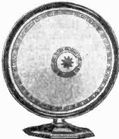
Trade Name—"Musicone"; Material of Horn—Paper Cone (specially treated); Finish—(Metal Parts) Bronze, (Cone) Mottled Brown; Type of Magnet—Crosley Patent; Action—Crosley Patented Magnetic Movement; Height—13½ in.; Diameter of Cone, 11½ in.; Weight—2¾ lbs.; Price—\$17.50.
