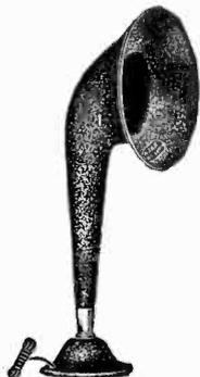
Trade Name—"Ajax Marveltone"; Material of Horn—Hard Rubber; Finish—Black; Type of Magnet—Horseshoe; Action—Coil, Adjustable; Control—Thumb Screw in Base; Height—17 in.; Diameter of Bell, 10 in.; Weight—8 lbs.; Price—\$15.00 list.
