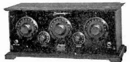
Trade Name—"Standardyne"; Type—Tuned Radio Frequency; Tubes—5; Battery—"A" Storage; "B" 90 Volts; Control—Tuning, 3; Tube, 2; Dim.—20 x 9 x 8¾; Wt.—15 lbs.; Price—\$60.00.
