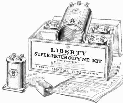
This comprises a special in-pot transformer, three intermediate wave transformers, one oscillator pick-up coil, one .0005 mfd. by-pass condenser, and a set of construction prints, diagrams, and data.
