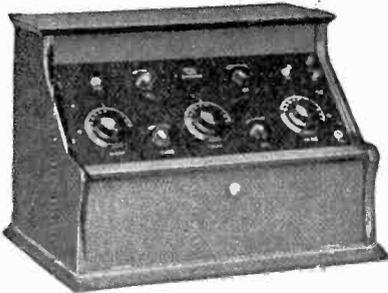
Trade Name—"Superfive"; Type—Radio Frequency; Tubes—5; Battery—"A" Storage or Dry; "B" 90 Volts; Controls—Tuning, 3; Tube, 3; Antenna—Loop, Indoor and Outdoor; Dim.—15½ x 22¼ x 15¼; Wt.—22 lbs.; Price—\$180.00.
