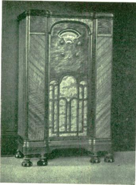
ALL WAVE —Model 318K—8-tube superheterodyne with 9 tuned circuits—complete world-wide range from 540 kilocycles to 22.5 megacycles—in 4 separate tuning bands—2-speed tuning, approximately 6 to 1 and 60 to 1 ratios—shadow tuning—six watts output—11-inch electro-dynamic speaker. Beautiful lowboy cabinet of choice veneers and matched woods with excellent acoustical properties. $89.90 f.o.b. factory.
