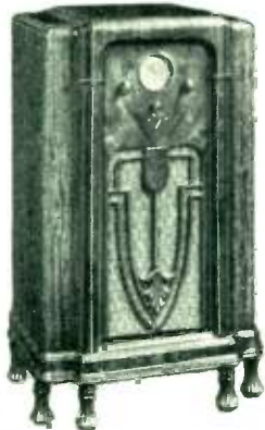
MODEL 752—7 tubes. Four band, truly all-wave set. 550 kilocycles to 21.7 megacycles. 10 inch Synchro-dynamic speaker.
