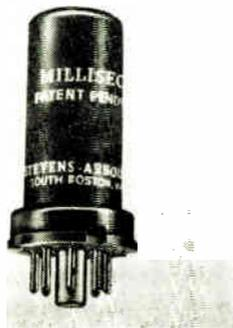
This Milliseo Relay has an operating time as short as 1/3 milliseconds; it is assembled in a metal radio tube container with an 8-prong octal base, but its operation is mechanical rather than electronic. Previously, these relays were made in one size only, but due to the demand for multiple pole construction, this firm is now offering these relays in the same container except double pole, double throw.
