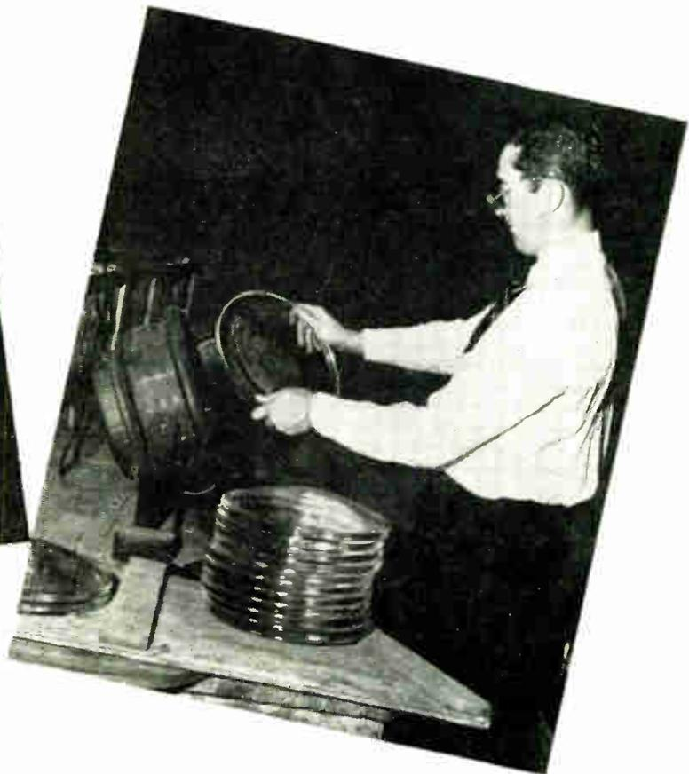
← Television screen images having six to seven times the illumination are being produced by a reflective type optical system using concave spherical glass reflectors, and play an important part in solving the problem of transmitting enough light from cathode ray projector tube to the screen. Made by McKee Glass Co., Jeannette, Pa.
