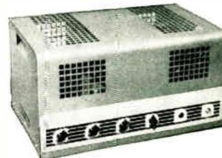
UNDERWRITERS' LABORATORIES APPROVED. Two microphone, one phono channel. Bass-Treble Tone Control. Response: 30-20,000 cps  $\pm$  1 db. Push Pull 807 constant voltage output. Oil filled filter capacitor, cable harness construction, safety interlock switch.
