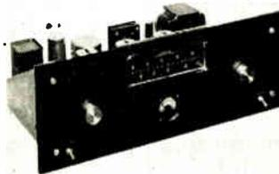
A new design standard broadcast (AM) tuning unit, with frequency coverage of from 550 to 1700 KC. A unique bridge-type balanced modulator employed in the superhet circuit is said to eliminate noise ahead of the IF amplifier, and cancels second order modulation products, which are the cause of most "birdies".
