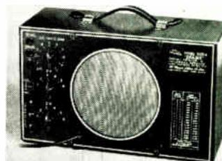
This model 905A "Sparx" is a super-sensitive aural dynamic signal tracer incorporating 18 watt universal output transformer and test speaker. Employs new vacuum tube hand-size probe on extra-flexible 4 foot cable. Frequency range of probe and cabinet-contained 2 stage a.f. is 20 cycles through 200 megacycles for AM, FM
