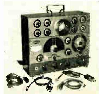
This device makes it possible for television and radio servicemen to make accurate alignments on all types of television and FM receivers. Called the Philco Model 7008, this is said to be the only complete portable instrument in its field, and contains the following: a crystal calibrator, to provide accurate check points every five megacycles; an AM (marker) generator; an FM generator; a special oscilloscope; and a common power supply.
