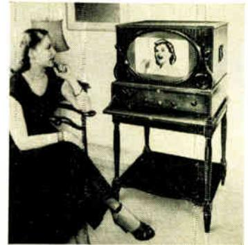
The "Sightmaster" screen (patents pending) becomes a decorative mirror when the set is not in use. When the set is in operation the picture appears on the mirror itself. It is not a reflected image, but a picture actually transmitted through the mirror. Purpose behind the mirror is to overcome the necessity of the unattractive blank television screen when the set is not in use. The receiver employs a 15" tube and also combines continuous tuning on FM radio.
