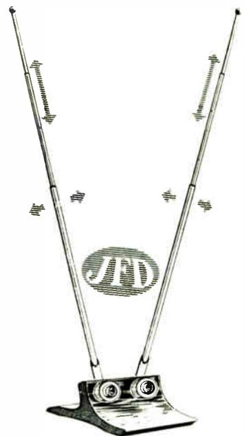
Featuring a marblette base in jade green or walnut, this indoor television FM antenna weighs less than a pound and a half. Telescopic dipoles are adjustable for all TV channels and for FM reception. Preassembled for immediate installation, it has a 10-foot length of 300-ohm twin lead. Say you saw it in *Radio & Television Journal*, June, 1949
