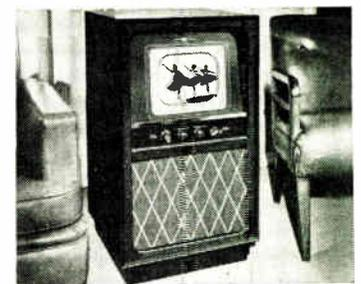
Model 809 television console features the GE "daylight" tube. Has 17 tubes and three rectifiers, plus 10-inch picture tube. Compact contemporary console is finished in mahogany. Pre-tuned to 12 TV channels, has automatic clarifier, and stabilization circuit for picture clarity and sharpness.
