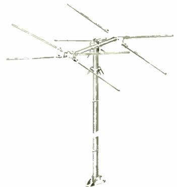
A conical-type Redi-Mount TV aerial designed for fringe areas. Features hi-gain, with television coverage on all channels coupled with FM coverage. Stands seven feet when erected, has two mating mast sections, guy wire anchor, standoff pole insulators, and adjustable mounting base. Comes completely preassembled.
