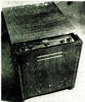
With 36 tubes, including picture tube, and six rectifiers, this chairside projection model in crotch mahogany throws a 3- by 4-foot picture on a home movie type screen. Cabinet measures 23 inches high, 21 wide and 26 long. Small doors in cabinet open to reveal the Proj-Tel unit, which houses projection system. Top slides forward to expose controls on back of cabinet. Set plugs into standard outlets, requires no special antennas. Say you saw it in *Radio & Television Journal*, June, 1949
