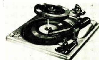
This three-speed changer will automatically play 10-, 12-, and 7-inch records at 33 1/3-, 45-, and 78-rpms. One spindle handles all three types of records, a collar centering the RCA 45-rpm records. Controls provide a speed selector lever, reject, manual control for automatic or manual playing. Tandem-Tip needle provides microground tip for microgroove records, and a standard ground tip for standard records, both on one needle.
