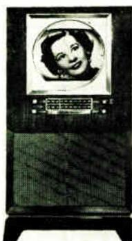
With a 10-inch cathode-ray tube producing a 61-square-inch picture, this console television set operates on channels 2 to 13 inclusive. Has 27 tubes, in addition to picture tube, and six rectifiers (four selenium). Automatic gain control circuit. FM sound channel. High-Q IF coils, tuned RF stage, and "Miracle" picture-lock. Also has Alnico V PM dynamic speaker. Cabinet comes in pin striped mahogany veneers.
