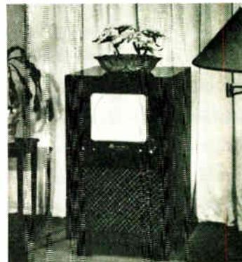
One of ITC's "Century" line of television receivers, this model has a 12½-inch cathode-ray tubes which gives an 85-square-inch picture. Eighteen tubes and three rectifiers; "Visual Tuning" and simplified controls. Available in cabinets of dark or bleached mahogany.
