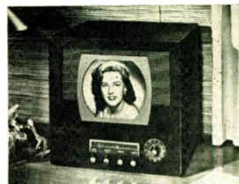
Total picture area of this television receiver which uses a 10-inch cathode-ray tube is over 62 square inches. Set has 25 tubes, plus three rectifiers, exclusive of picture tube. Channel selector tunes picture and FM sound simultaneously. Has gyromatic picture lock, four-stage IF amplifier, five tuned circuits, and automatic gain control. Cabinet in dark Honduras mahogany has recessed framing.
