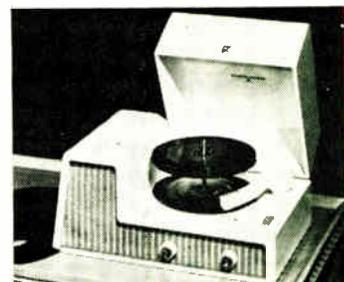
An automatic table model phonograph developed for playing Columbia and RCA 7-inch records automatically. Model 745 is a two-speed changer with velocity trip, 3-second cycle change "music to music," controlled tone arm performance, and non-record slippage. Housed in plastic, unit has self-contained amplifier and speaker.
