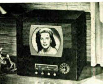
Total picture area of this television receiver which uses a 10-inch cathode-ray tube is over 62 square inches. Set has 25 tubes, plus three rectifiers, exclusive of picture tube. Channel selector tunes picture and FM sound simultaneously. Has gyromatic picture lock, four-stage IF amplifier, five tuned circuits, and automatic gain control. Cabinet in dark Honduras mahogany has recessed framing.
