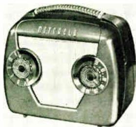
This radio weighs four pounds and operates from batteries only. Has specially designed Hi-Q IF transformers, cosmalite forms and silver mica capacitors for maximum performance and stability. Loop antenna is built into back of set.
